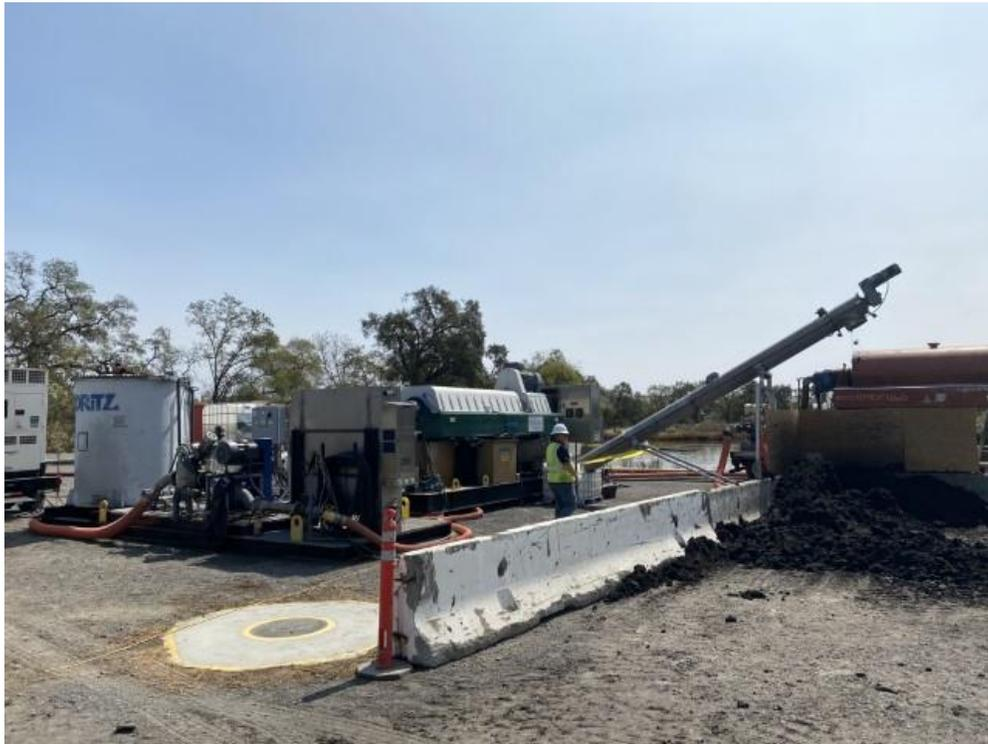
**Figure 2-5. On-site Mobile Dewatering Unit**
