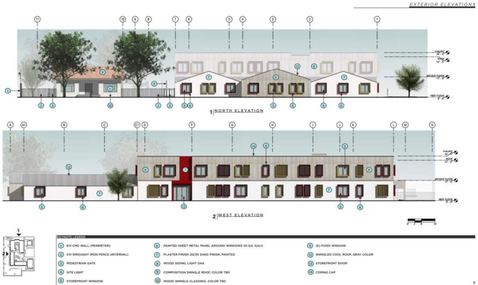
Figure 5 Project Elevations – North and West
