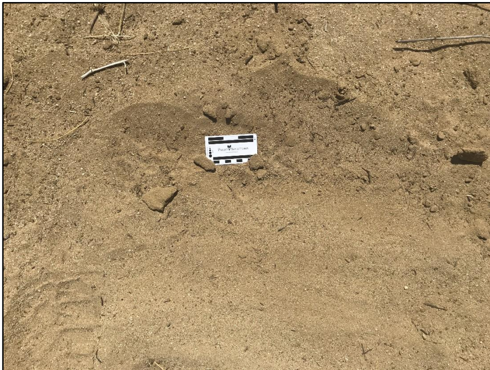
Figure 10. Photo taken from along the eastern portion of the Project area (solar field) and viewing toward the ground surface: exposed surficial sediments comprising Holocene-age young sand deposits (Qs) in an area mapped as Holocene-age young alluvium (Qa) (see Appendix B).
