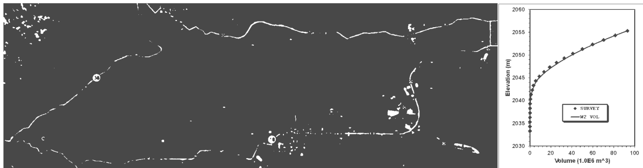
Figure 10. CE-QUAL-W2 model grid developed for Big Bear Lake. Inset depicts agreement between model and measured volume-elevation relationships.
