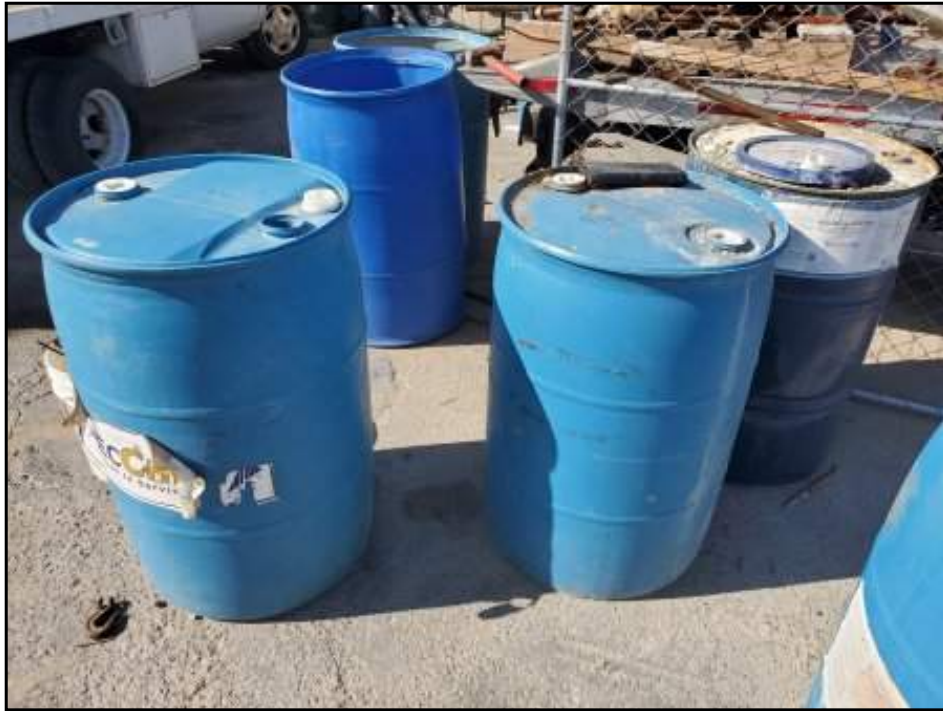
View of partially full drums of Spec Strip, a concrete form release agent observed in construction yard.
