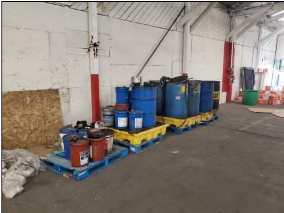
View of hazardous material storage including used oil and new oil in 745A E State St.
