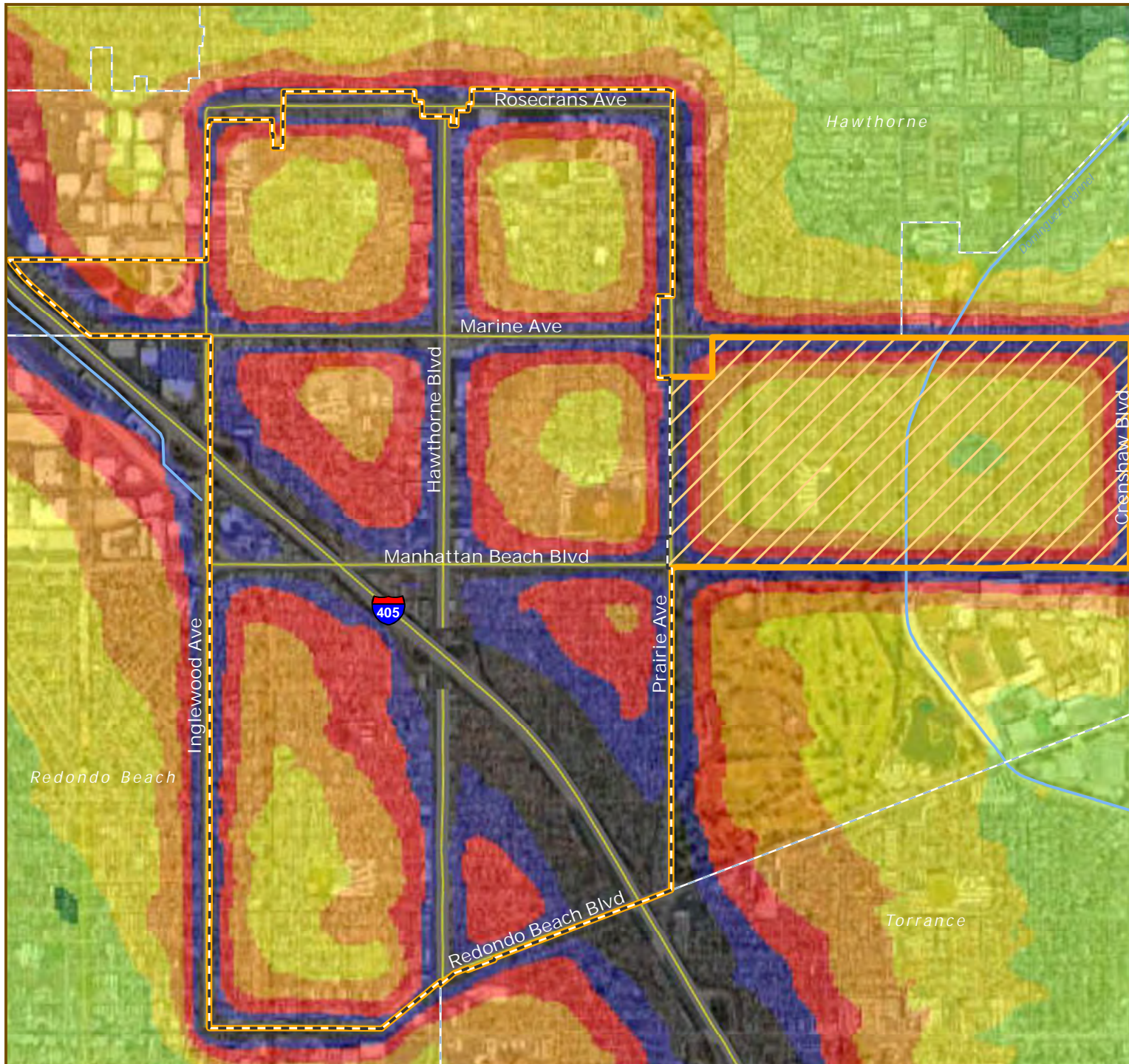
Figure 5.13-3. 2045 No Project Noise Level Contours
