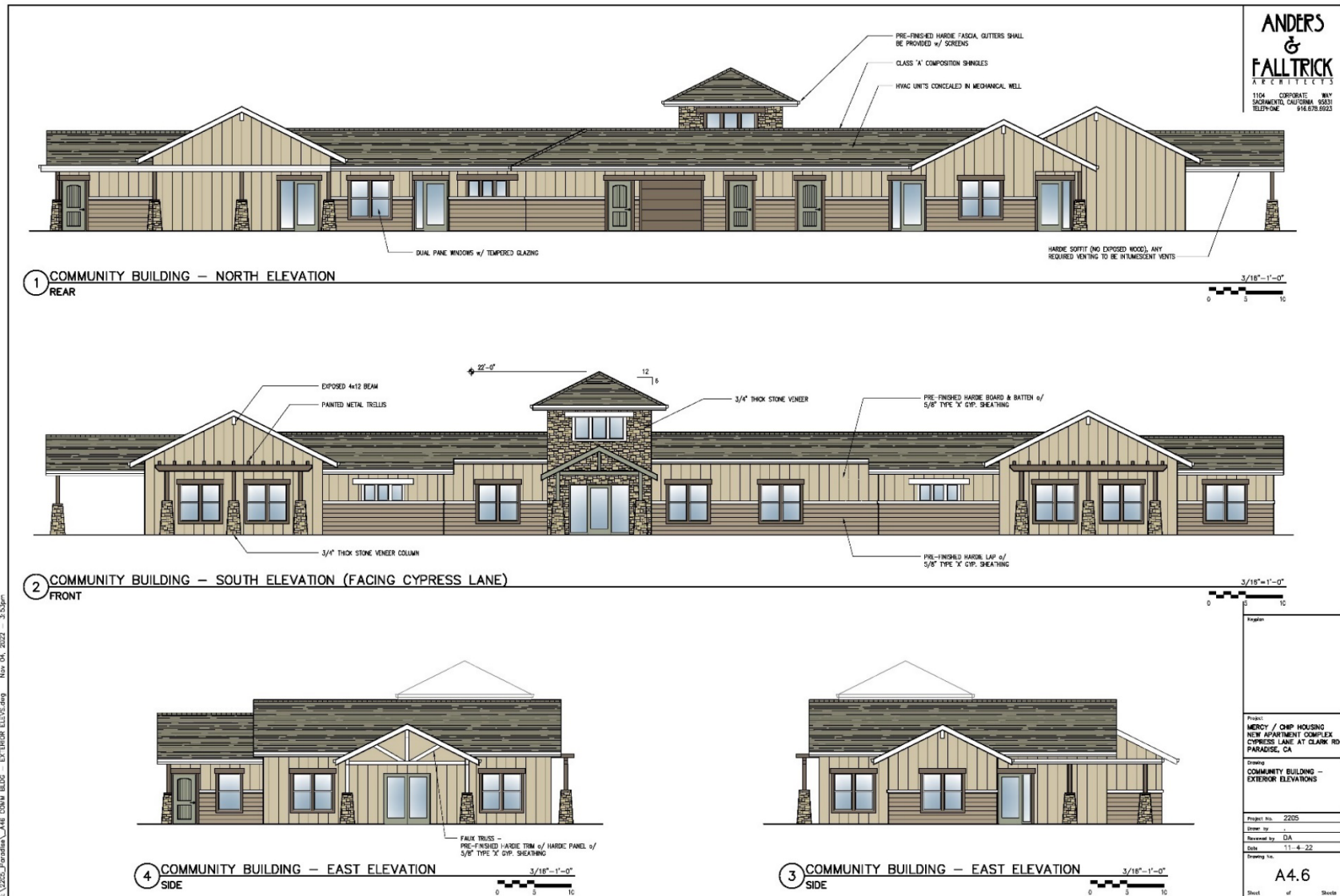
Figure 9. Community Building Elevations
