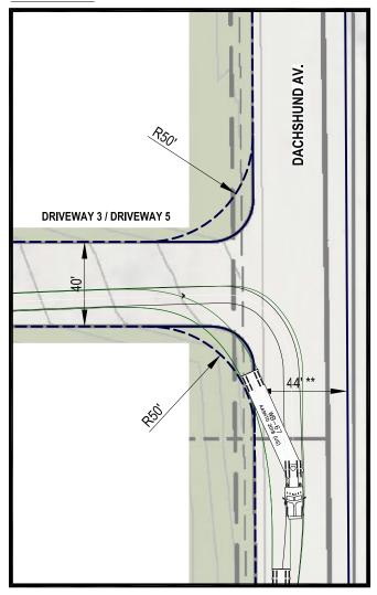
\*\* 44 FEET OUTSIDE CURB TO EASTERLY EDGE OF PAVEMENT IS EQUIVALENT TO THE HALF-SECTION PLUS ONE LANE IMPROVEMENT ON DACHSHUND AVENUE, ADJACENT TO THE SITE
