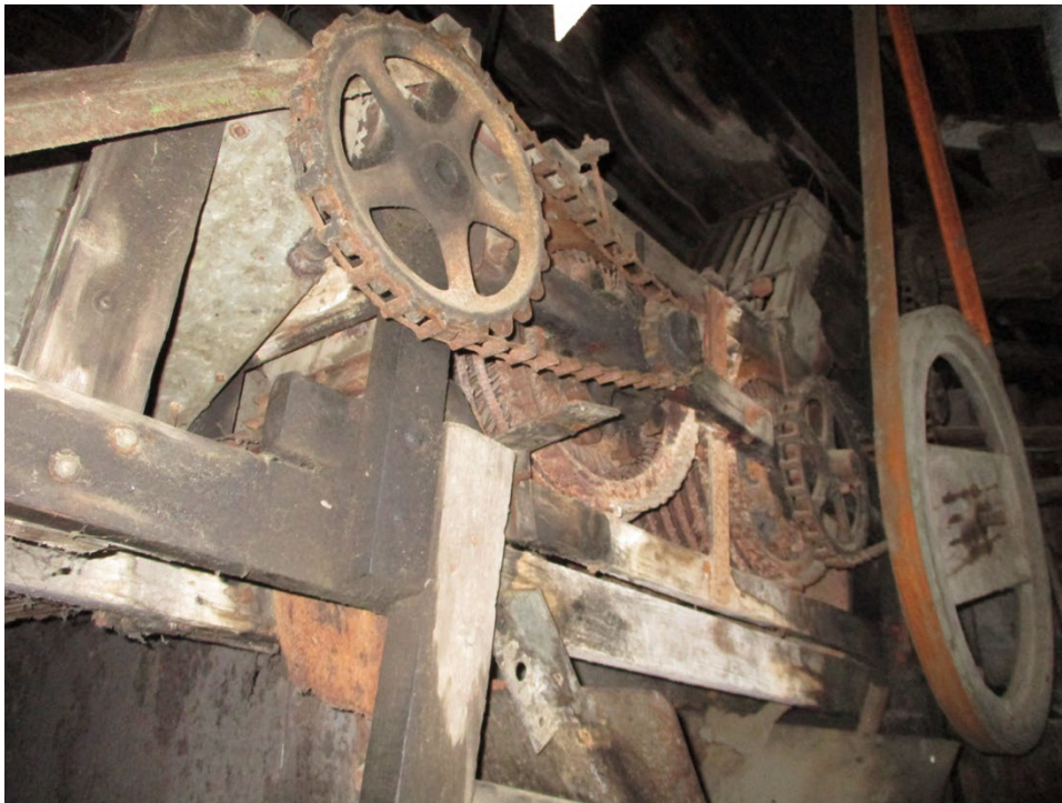
Figure 9. Mechanics of walnut conveyor belt.
