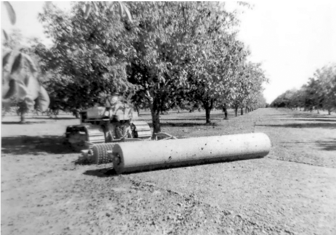
Figure 16. 1950s photograph of a D4 tractor pulling a drag ring-roller and smooth roller to prepare for walnut orchard harvest on Bishop Ranch (courtesy of San Ramon Chronicles: Stories of Bygone Days).
