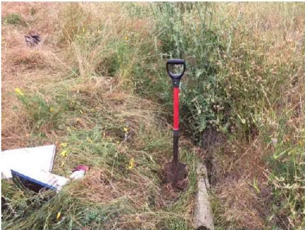
Appendix C-4. Man-made drainage ditch lacking an OHWM and positive indicators of all three wetland parameters at Sample Point 3.
