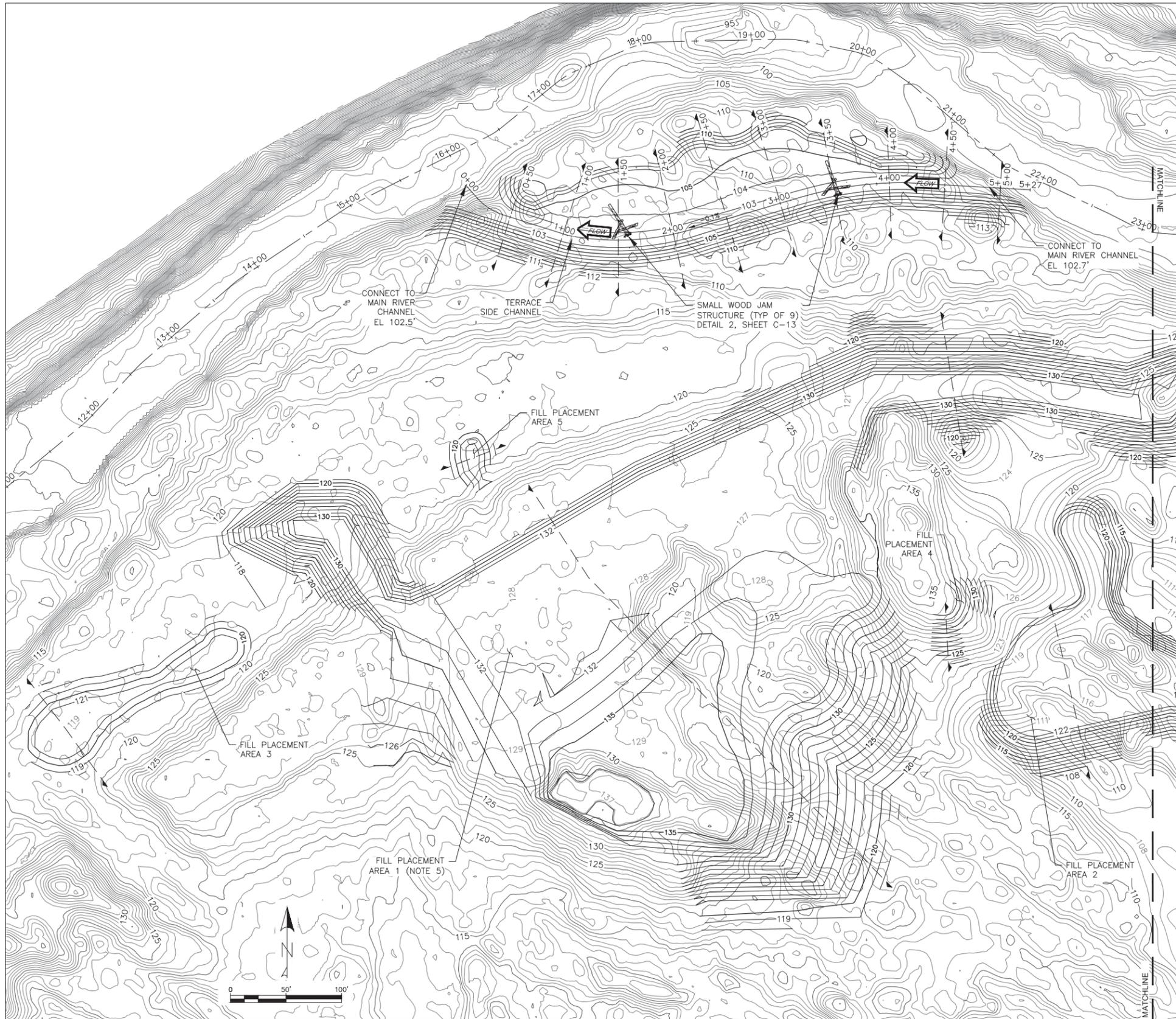
**GRADING PLAN - TERRACE SIDE CHANNEL & FILL PLACEMENT AREAS**
