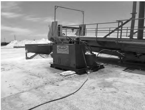
**Photo #23** View of the above ground hydraulic power source for the tipper containing diesel fuel and hydraulic oil.
