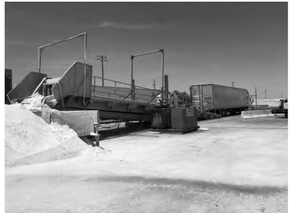
**Photo #22** View of the hydraulic truck tipper located on the central portion of the site.
