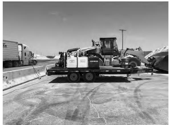
**Photo #24** View of a service trailer with air compressor, diesel, hydraulic oil and motor oil located east of the tipper.
