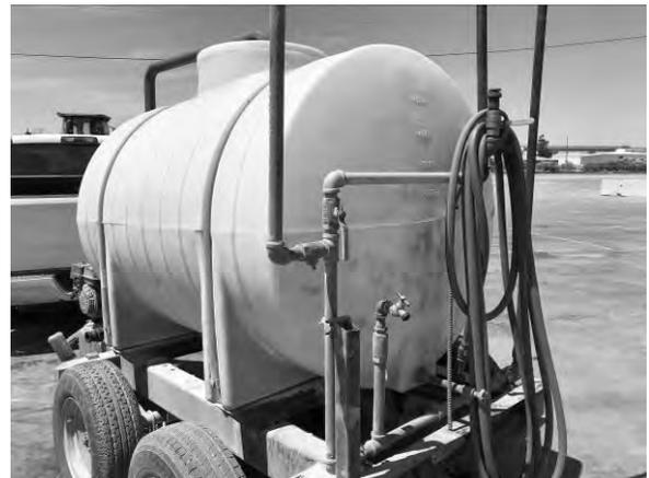
**Photo #12** View of a 500-gallon container of water used for dust suppression.
