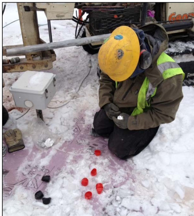
Figure 4. Removal and Capping of Sleeved Samples
