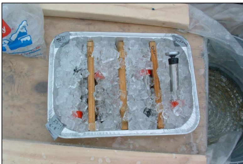
Figure 5. Ice Bath for Cooling Samples
