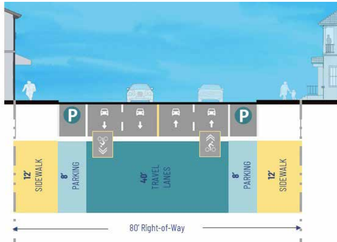
Figure 3.6 Main Street Existing Road Section
