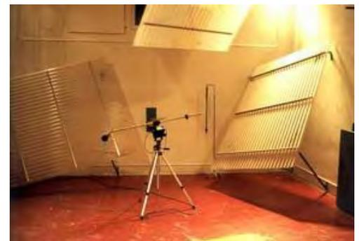
Figure 12. Barrier absorption: Reverberation Room Method
