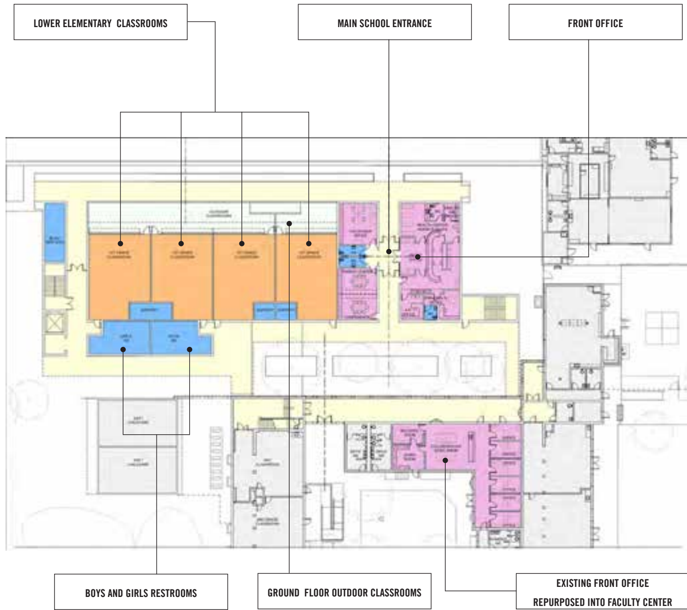
PROJECT 1 NEW CLASSROOM BUILDING GROUND FLOOR Four elementary classrooms with associated outdoor classrooms, front office and school support
