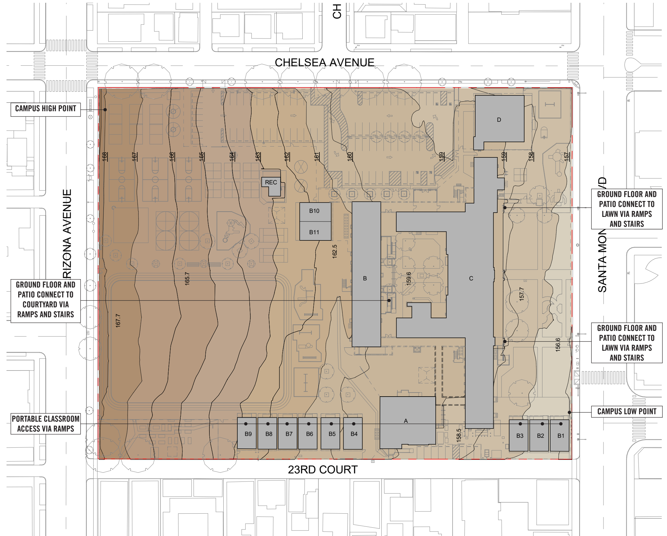
TOPOGRAPHY Campus elevations vary across the site by approximately eleven feet. Localized differences are mitigated by ramps and stairs to provide access to campus buildings.
