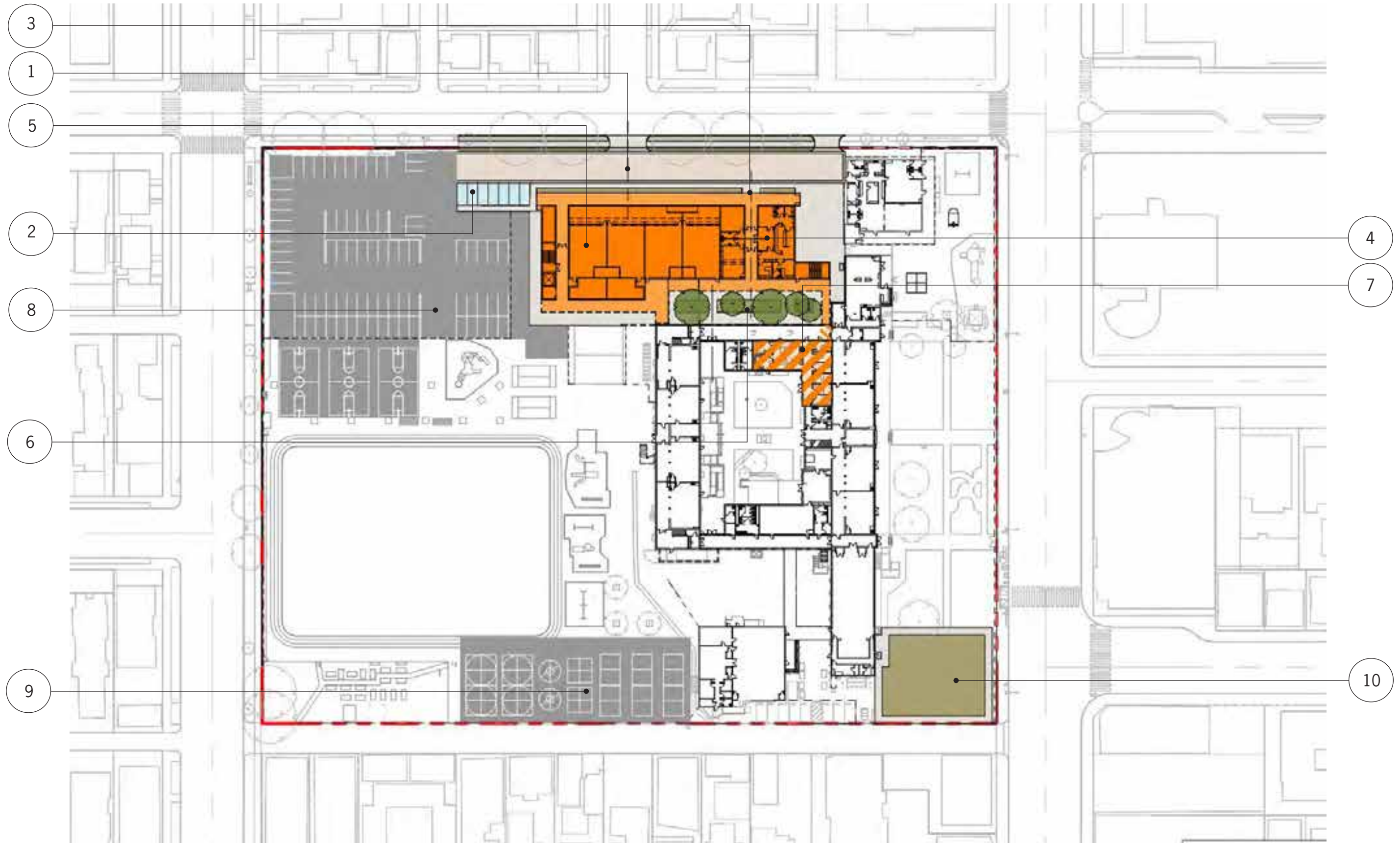
PROJECT 1: NEW CLASSROOM BUILDING FRONT OFFICE AND SCHOOL SUPPORT The new building creates a courtyard between it and the historic main building. The existing front office is repurposed into a new faculty center
