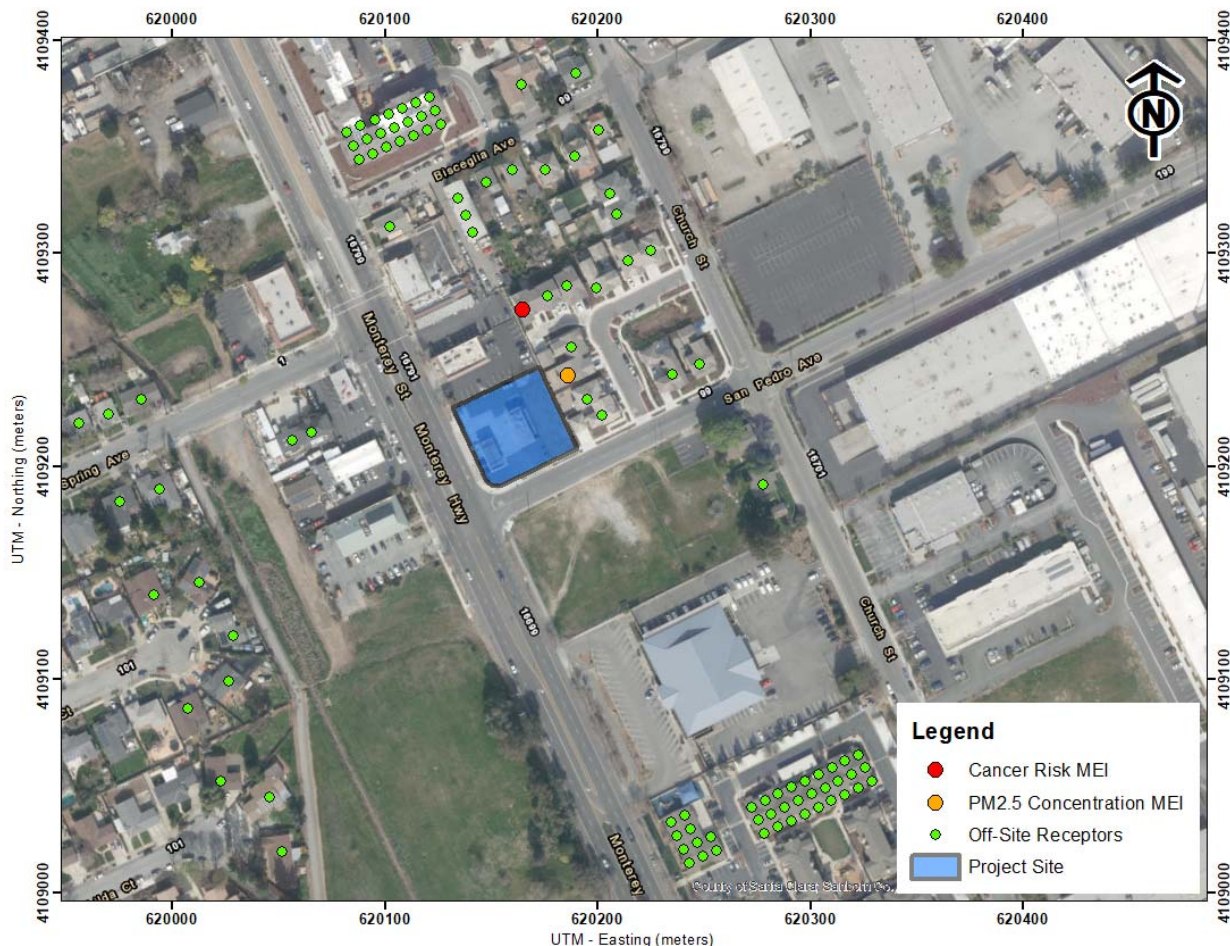
Figure 1. Project Construction Site, Locations of Off-Site Sensitive Receptors and Maximum TAC Impact Locations (MEI)
