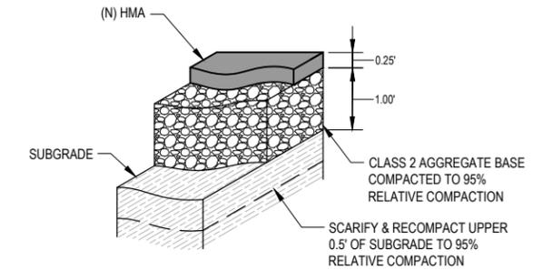
TYPICAL PAVEMENT STRUCTURAL SECTION DETAIL
