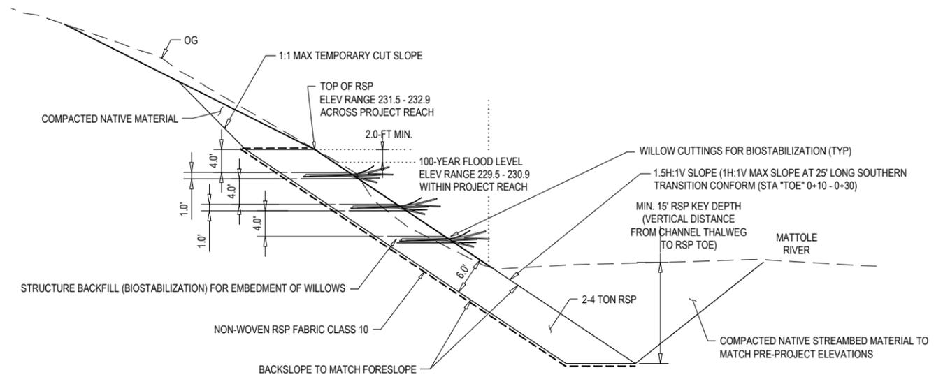
**TYPICAL SECTION STREAMBANK BIO-STABILIZATION SECTION**
