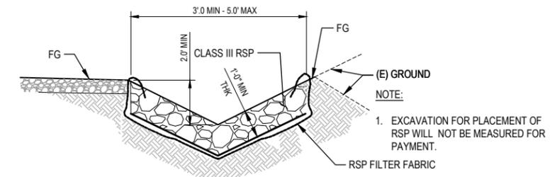
TYPICAL ROCK-LINED DITCH DETAIL (ROADSIDE)
