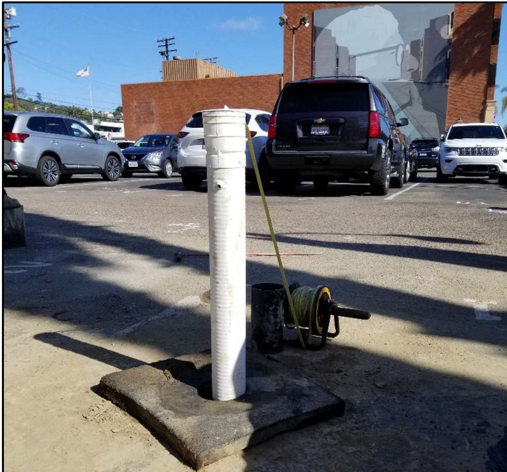
Figure 3-3. Percolation Testing at Boring P-2
