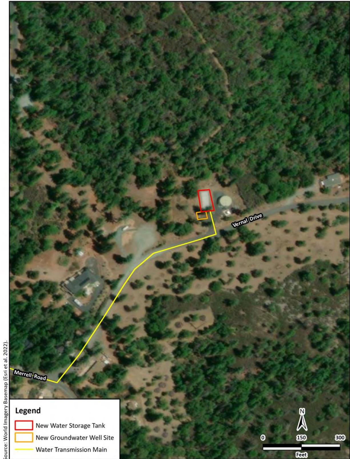
Figure 3 – Water Distribution Pipeline Site Map
