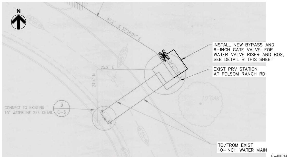
**EXISTING PRV STATION BYPASS PLAN**
