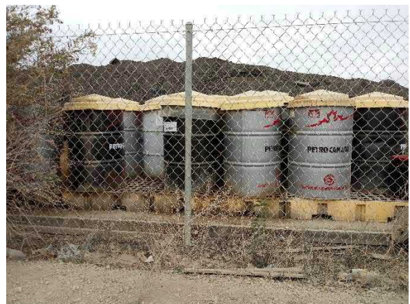
Photo #48 55-gallon drums on secondary containment located on the American Asphalt facility, and adjacent to the site boundary.
