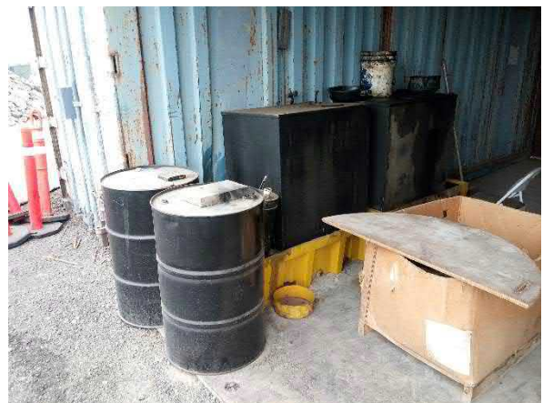
Photo #30 55-gallon drums containing methanol and two approximately 100-gallon ASTs with unknown contents located inside the Mike Bubalo staging area.
