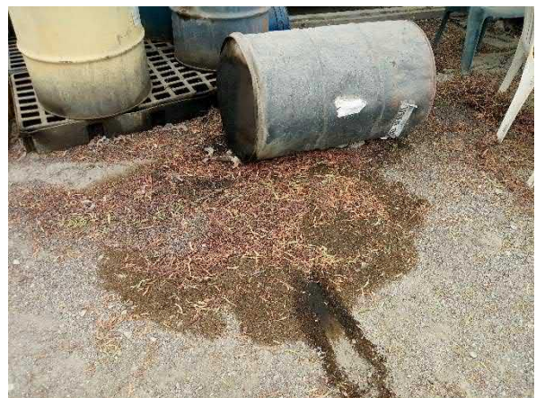
Photo #36 Soil staining emanating from a 55-gallon drum containing used oil, located near the landfill entrance.
