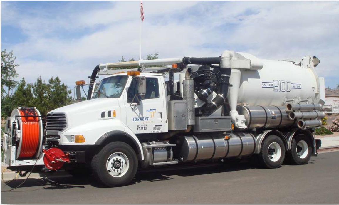
Typical hydro-vacuum truck used for drywell maintenance
