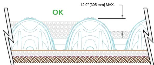
NOTE: STONE HEIGHT IN BETWEEN ROWS AND PERIMETER SHOULD NOT DIFFER BY MORE THAN 12" (300 mm).
