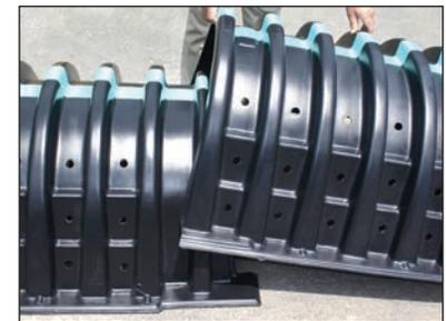
*Directional arrows located on the top of the chamber point towards the Small Rib End. The open end of the next chamber overlaps the small rib end of the preceding chamber.*
