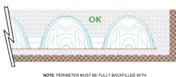
NOTE: PERIMETER MUST BE FULLY BACKFILLED WITH STONE AND EXTEND TO THE EXCAVATION WALL.
