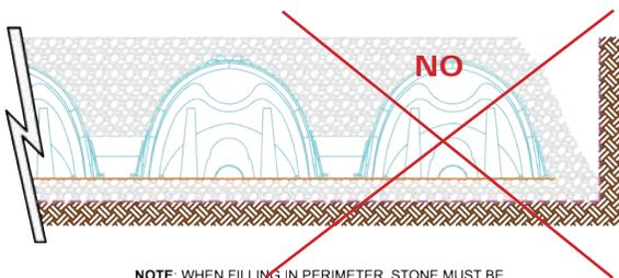
NOTE: WHEN FILLING IN PERIMETER, STONE MUST BE FILLED IN EVENLY WITH CHAMBER ROWS.
