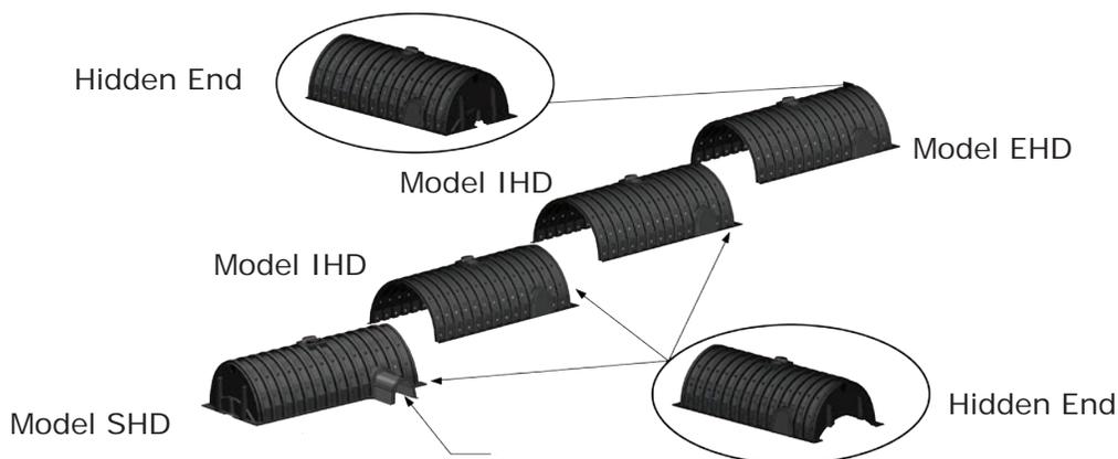
Shown with side portal trimmed and optional CULTEC HVLV Feed Connector inserted.
