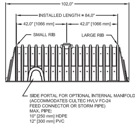
CULTEC RECHARGER 330XLHD CHAMBER STORAGE = 7.459 CF/FT [0.693 m³/m]
