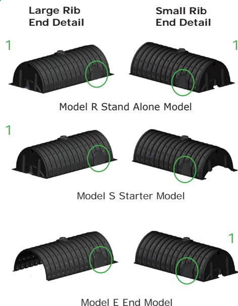
Trimming may only be performed on fully closed end walls (indicated by Number 1 in Fig. 1) or side portal areas (See green circles in Fig. 1 for side portal locations). Pipe may not be inserted into the sidewall of the chamber unless it is within the side portal trim lines. See page 11-12 for more information on trimming side portals.
