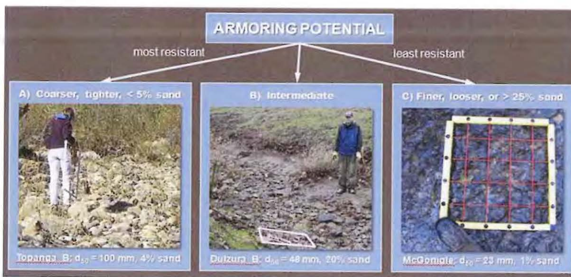
Figure 2.3: Armoring potential photographic supplement for assessing intermediate beds ( 16 < d_{50} < 128 mm) in conjunction with Checklist 1
