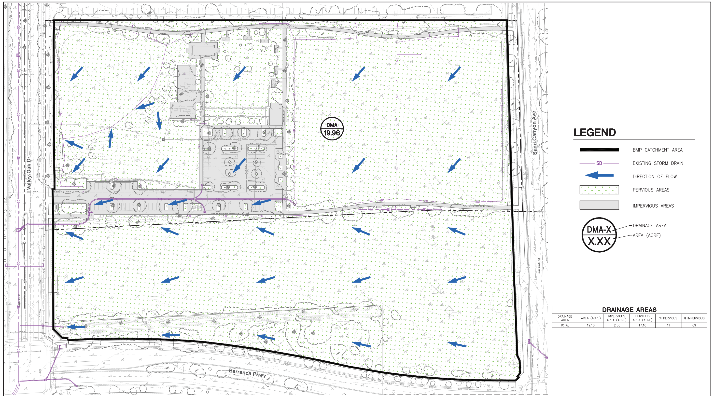
Figure 7 - WQMP Exhibit - Existing Conditions
