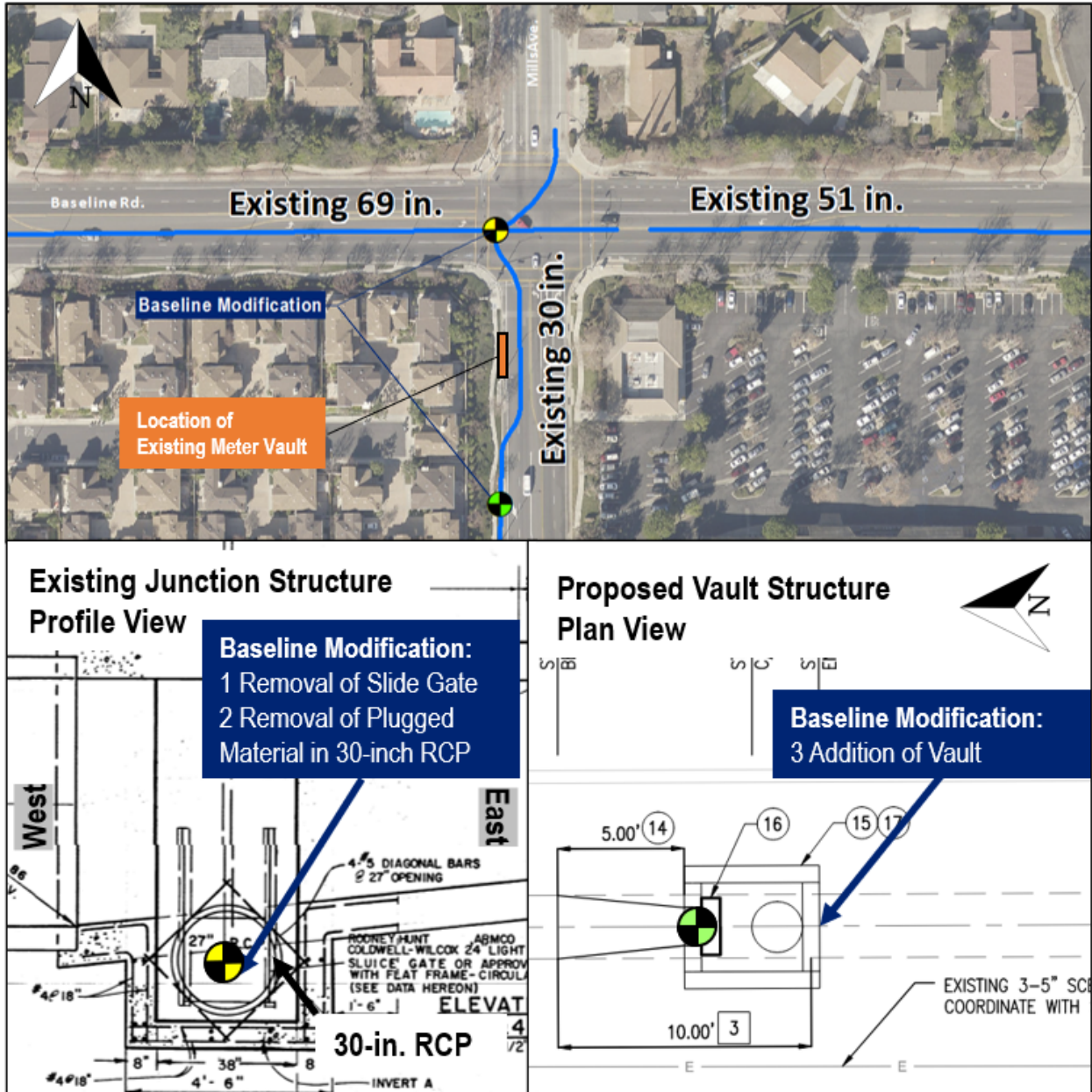
Figure 3. Proposed Storm Drain System Improvements
