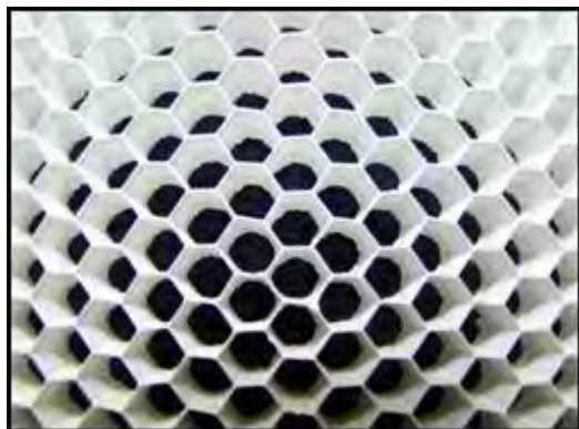
Close-up of the coated honeycomb matrix.
