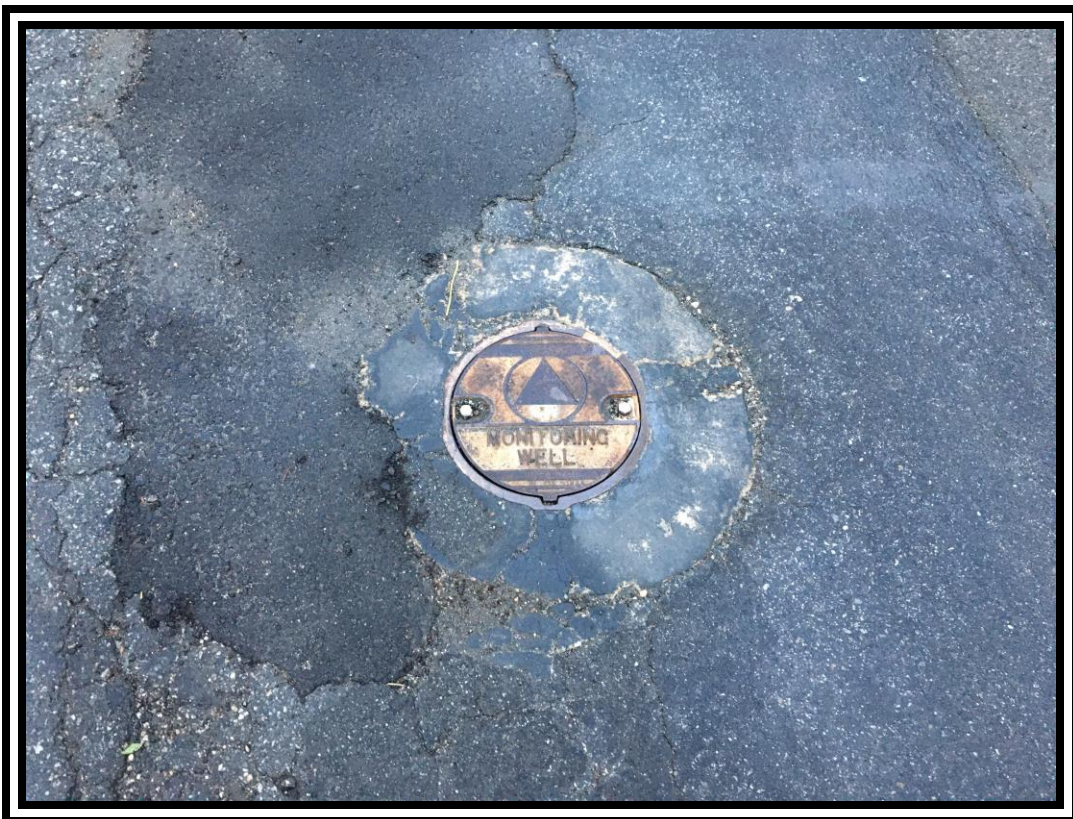
22. GROUNDWATER MONITORING WELL MW-8 IN ADJACENT WEST ALLEY, ASSOCIATED WITH ARCO CASE LOCATED ADJACENT EAST OF PROPERTY.
