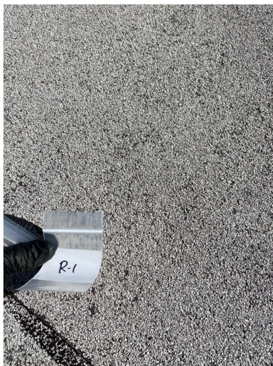
Picture 6: Rolled roofing sampled was found to not contain asbestos
