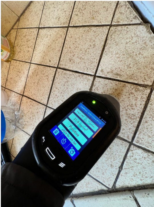
Picture 3: XRF detected lead-based paint on Unit H kitchen countertop tile of 6016 Norwalk Blvd. Whittier
