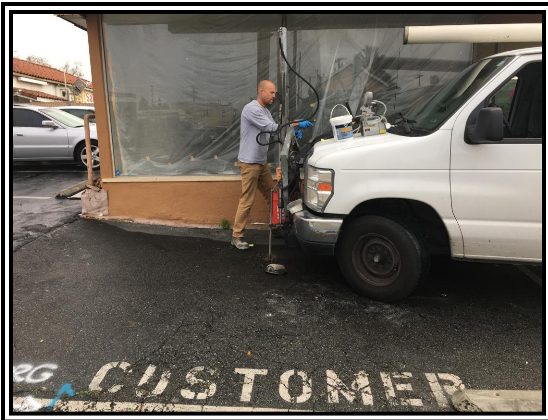
5. ADVANCING PROBE LOCATION SV-4 OUTSIDE NORTHERN AREA OF UNIT.
