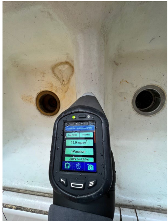
Picture 4: XRF detected lead-based paint on Unit H kitchen sink of 6016 Norwalk Blvd. Whittier
