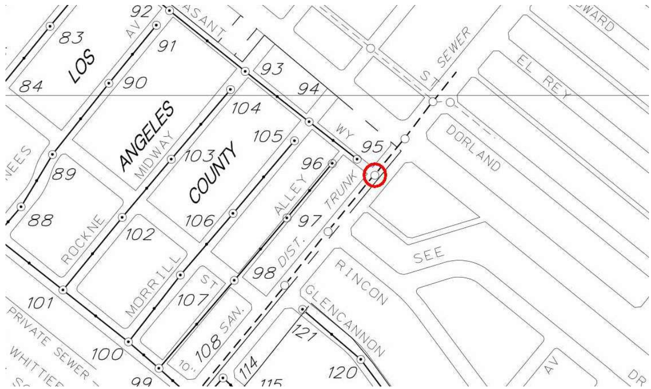
Figures 1 & 2: The vicinity map (above) shows the temporary wastewater flow monitoring location northeast of the proposed project site. The manhole is located at latitude 33.989530 and longitude -118.064406. A plan view of the monitored sewer line from CSMD C-2076 is shown below.
