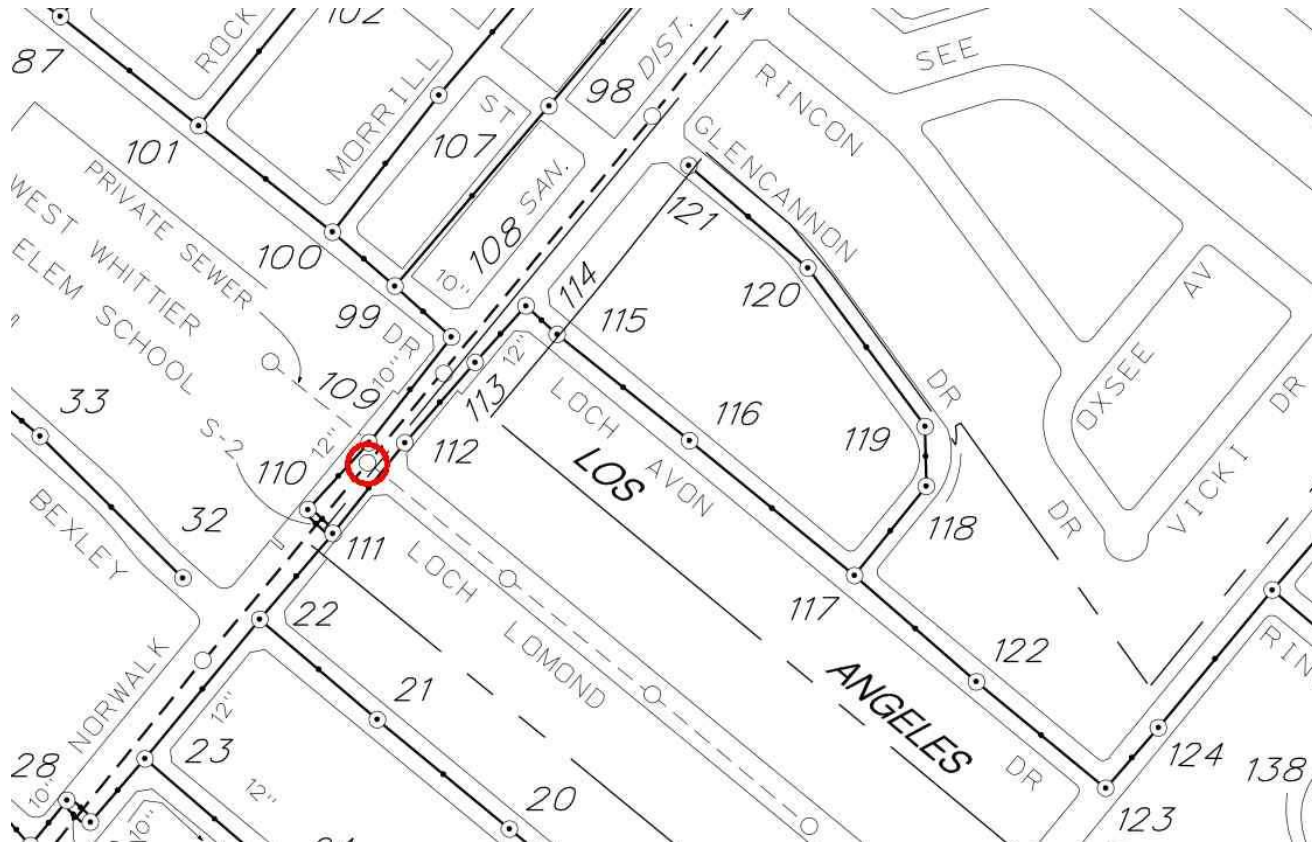
Figures 3 & 4: The vicinity map (above) shows the temporary wastewater flow monitoring location of City manhole (MH) 20, which is located at latitude 33.986733 and longitude -118.067174. A plan view of the monitored sewer line from CSMD C-2076 is shown below.
