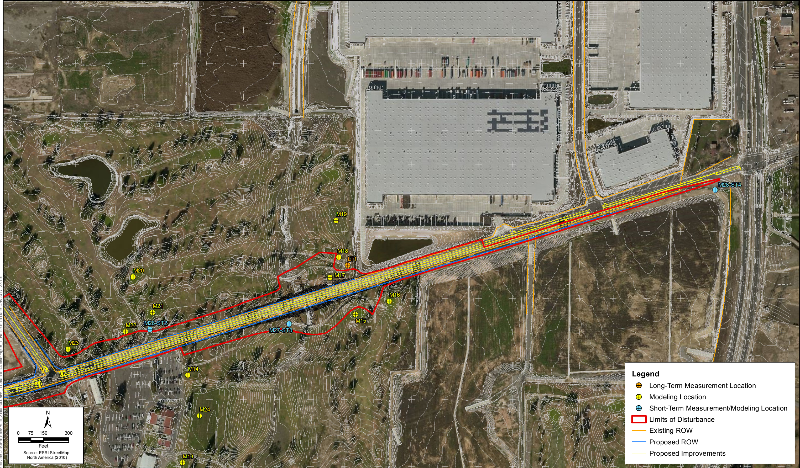
Figure 7 - Sheet 2 Noise Measurement and Modeling Locations Pine Avenue Extension Project
