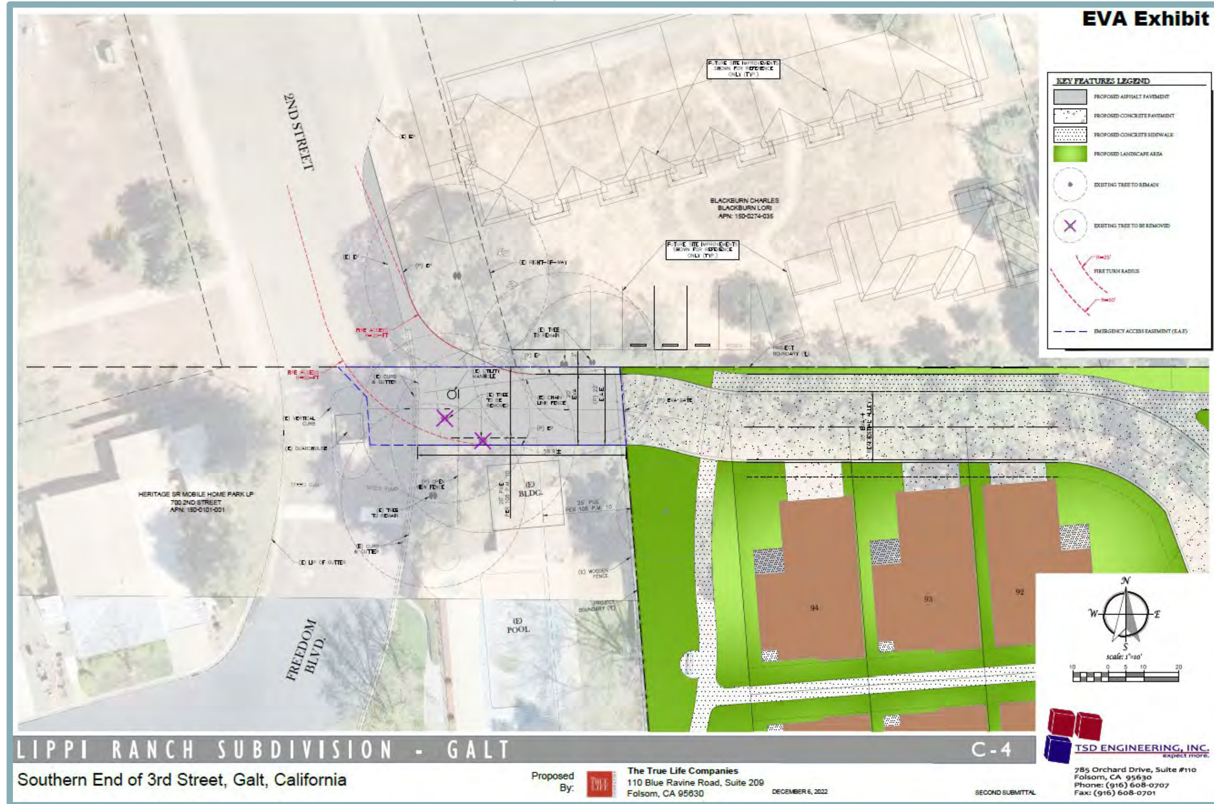
Figure 6 Emergency Vehicle Access Exhibit
