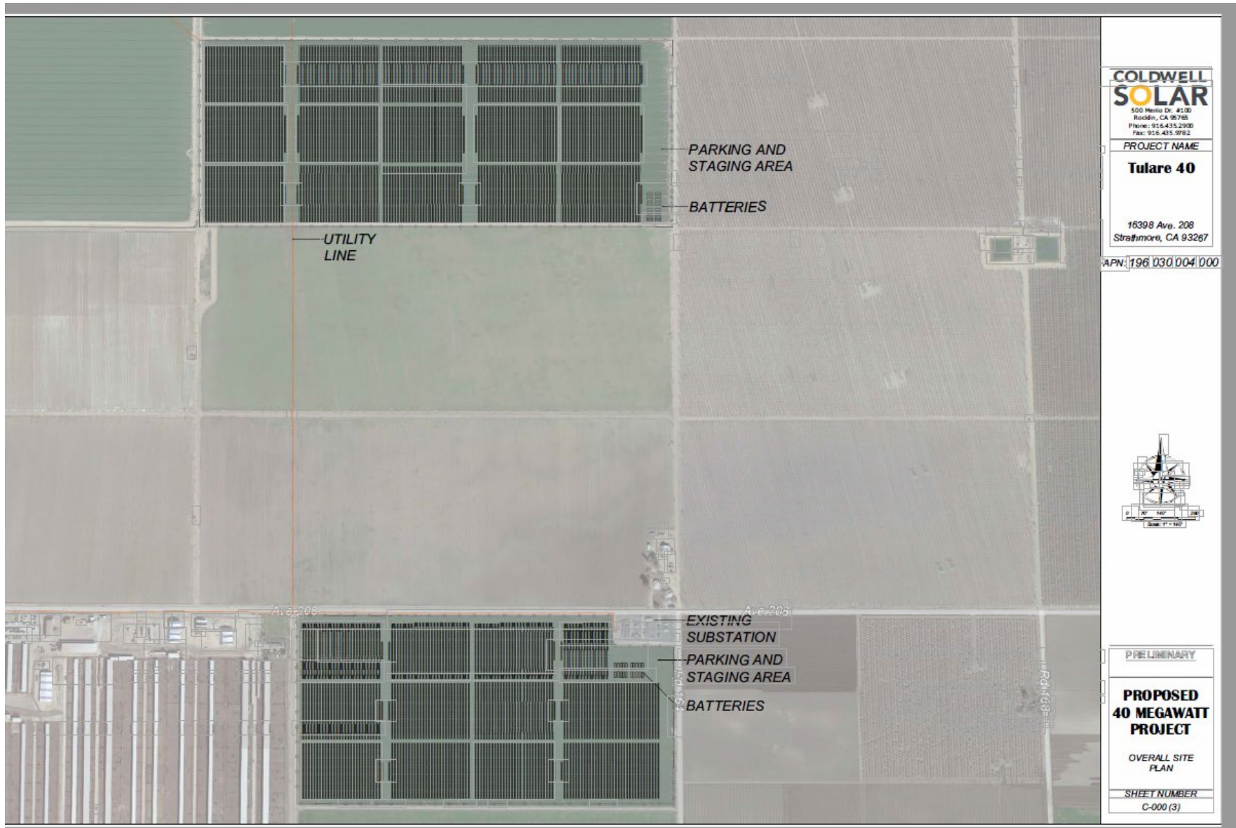
Figure 4 Site Plan North and South Arrays
