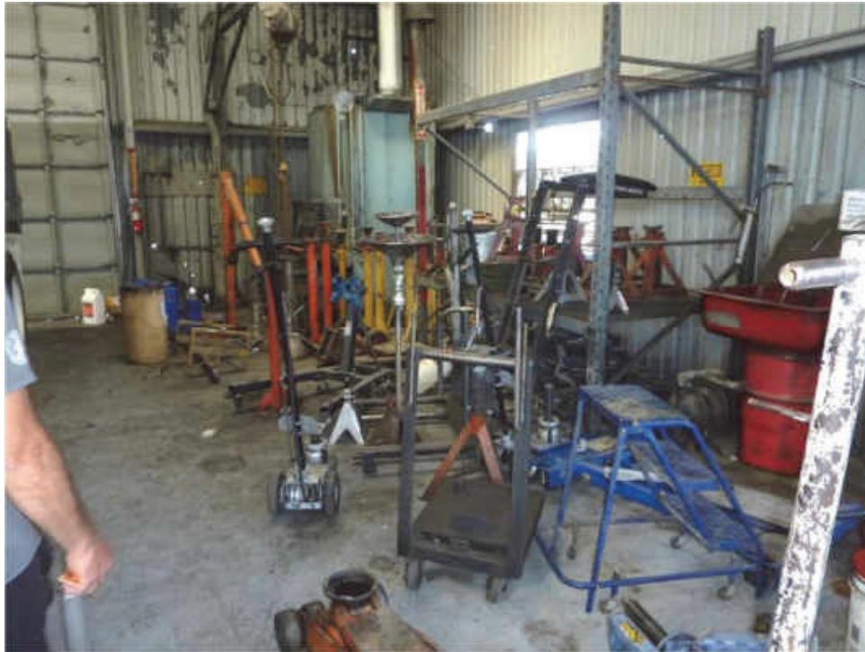
E-13. Looking at northwest corner of maintenance shop at 1535 Industrial Avenue with tub-type parts washer at right and enclosed spray cleaner in far background (06/22/2020).
