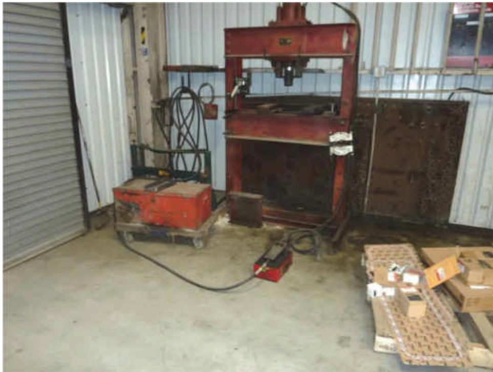
E-34. Hydraulic press inside northwest corner of truck repair shop at 1535 Industrial Avenue with oily residue on floor beneath (06/22/2020).
