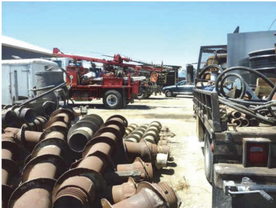
E-52. Looking southwest at drilling rigs and hollow-stem augers in Exploration Geoservices yard at 1575 Industrial Avenue, although address may be 1591 Industrial Avenue (06/22/2020).
