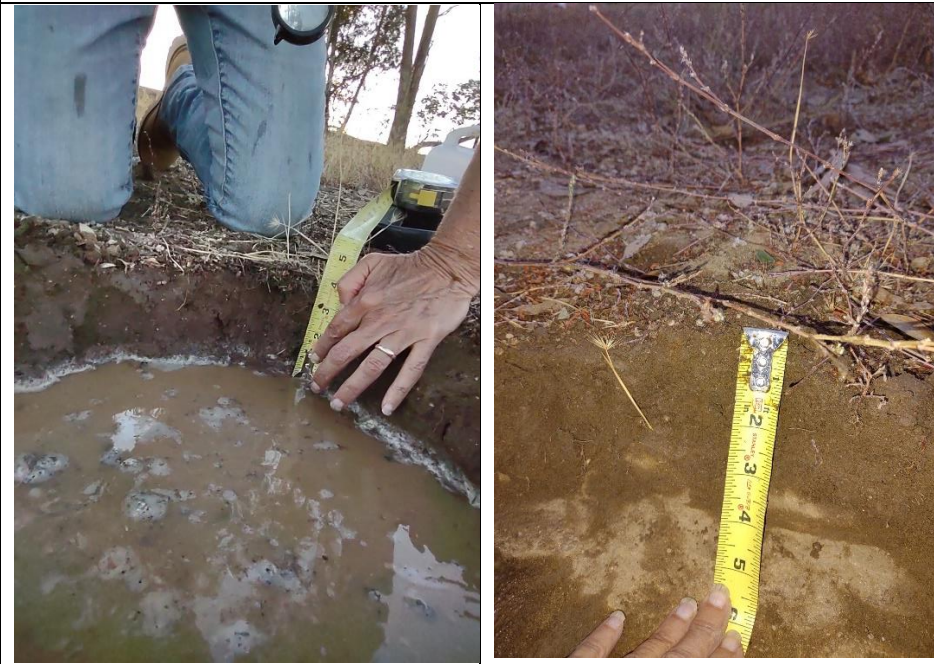
Fig 17. 08/11/2022 (Left) Pool 2. The soil was very hard and dry and had to be wetted to dig. Infiltration was very slow. By continuing to add water, I was able to dig a hole four inches deep to the boundary of the water impermeable layer. (Right) Scooping out the mud and breaking through the duripan to 6 inches it is evident that water perches at 4 inches.
