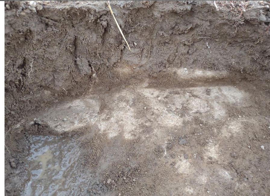
Fig 14. 08/11/2022 Pool 2 Soil profile with whitish top of silica-indurated layer of exposed and cleaned. The top 4 inches of the profile has a consistent matrix color without "redox" mottles. This soil failed the hydric soil test because it is not saturated long enough to develop the redox mottles. The water impermeable layer did not effervesce in acid. The soil is not alkaline.
