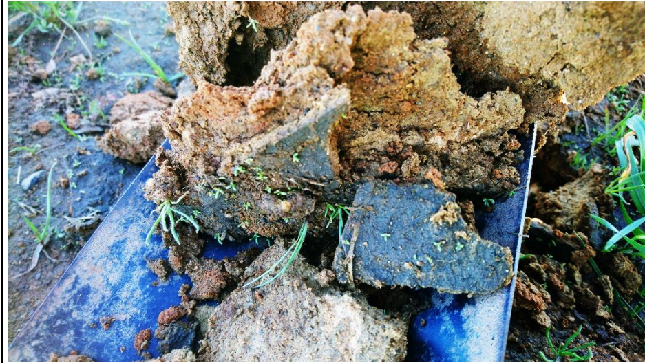
Fig 13. 11/28/2021 Soil from pool 1 on shovel blade after the first rain of the season. Note the thin dark surface coating which is a "biotic crust" of algae and silt that forms as a result of inundation. The 0-4 inch horizon has "distinct" oxidized mottles easily meeting the 5% or more requirement of "distinct" or prominent redox concentrations, at least 2 inches thick, within the top 6 inches of soil"
