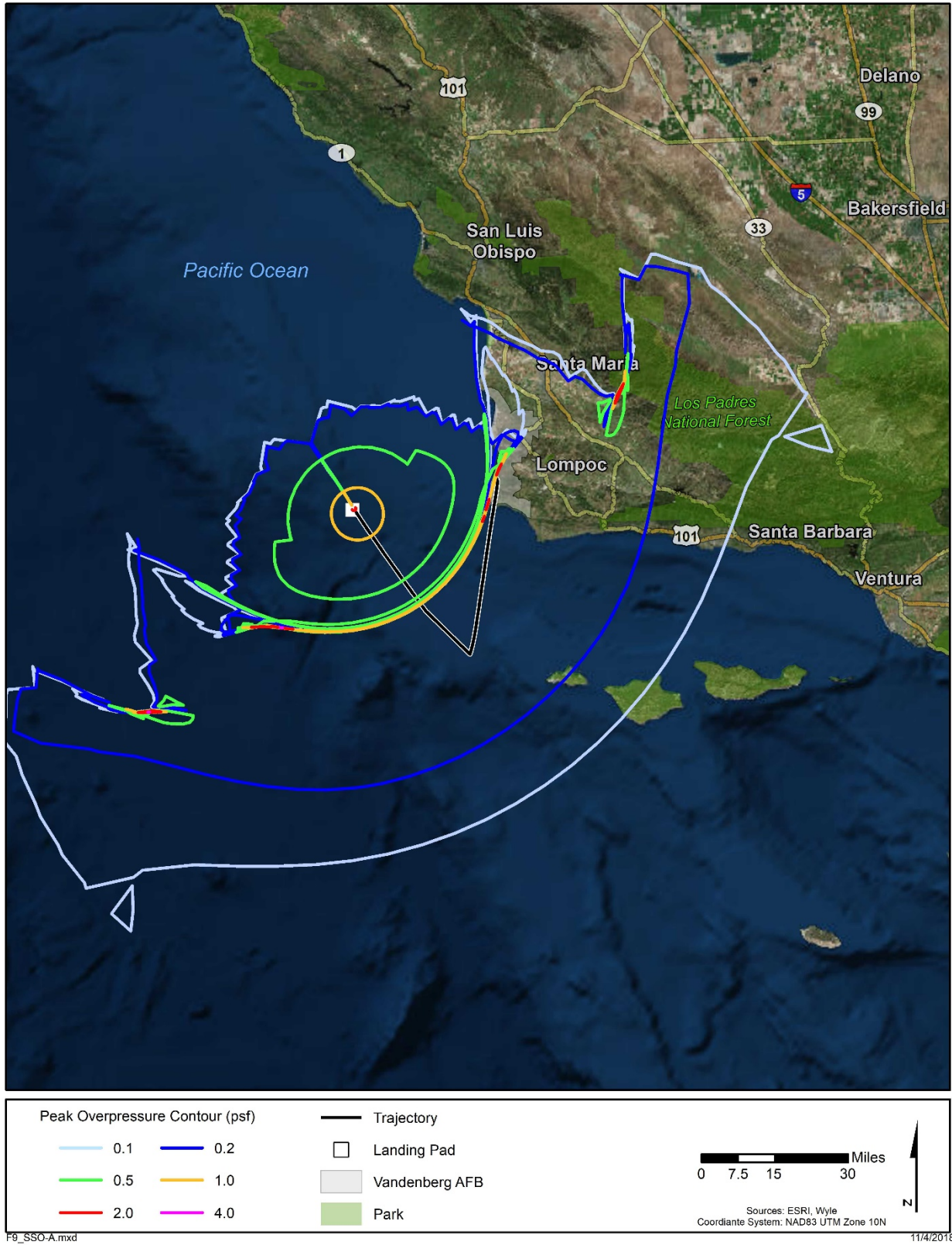
Figure 2.2-5. Sonic boom modeling results for first stage landing at an offshore droneship near VSFb for the Falcon 9 SSO-A mission.
