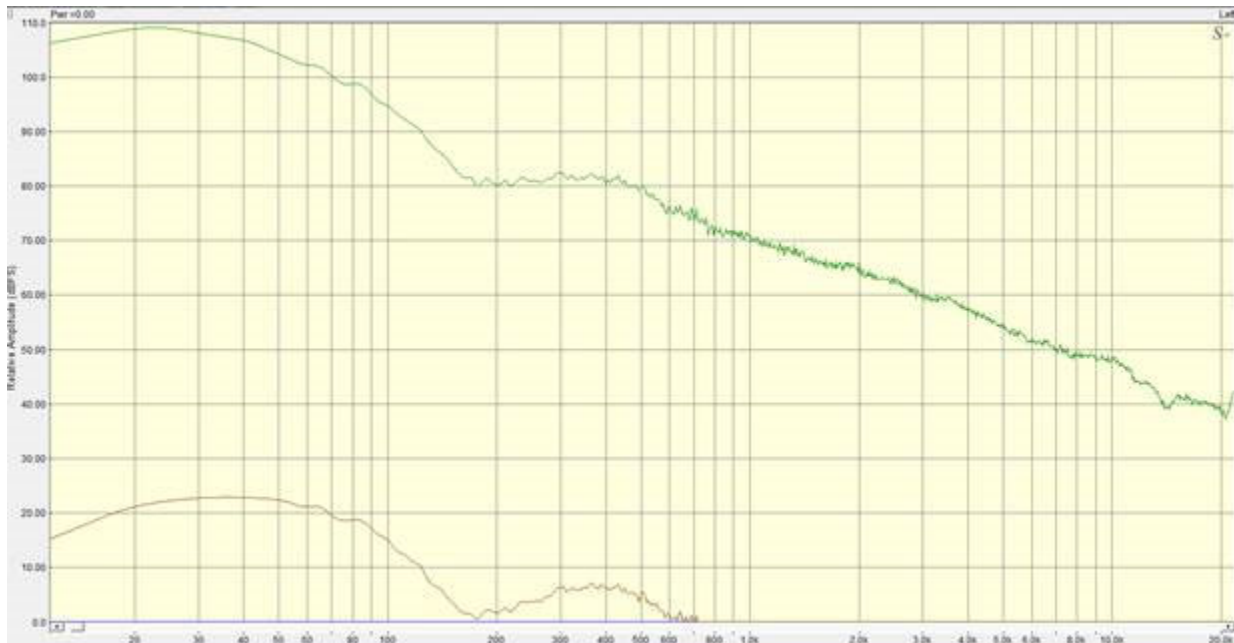
Figure 5.1-3. Launch peak noise level comparison of unweighted (green) versus Ranidae-weighted (brown) decibels (note: time waveform recording from the June 2022 Falcon 9 SARah-1 launch).
