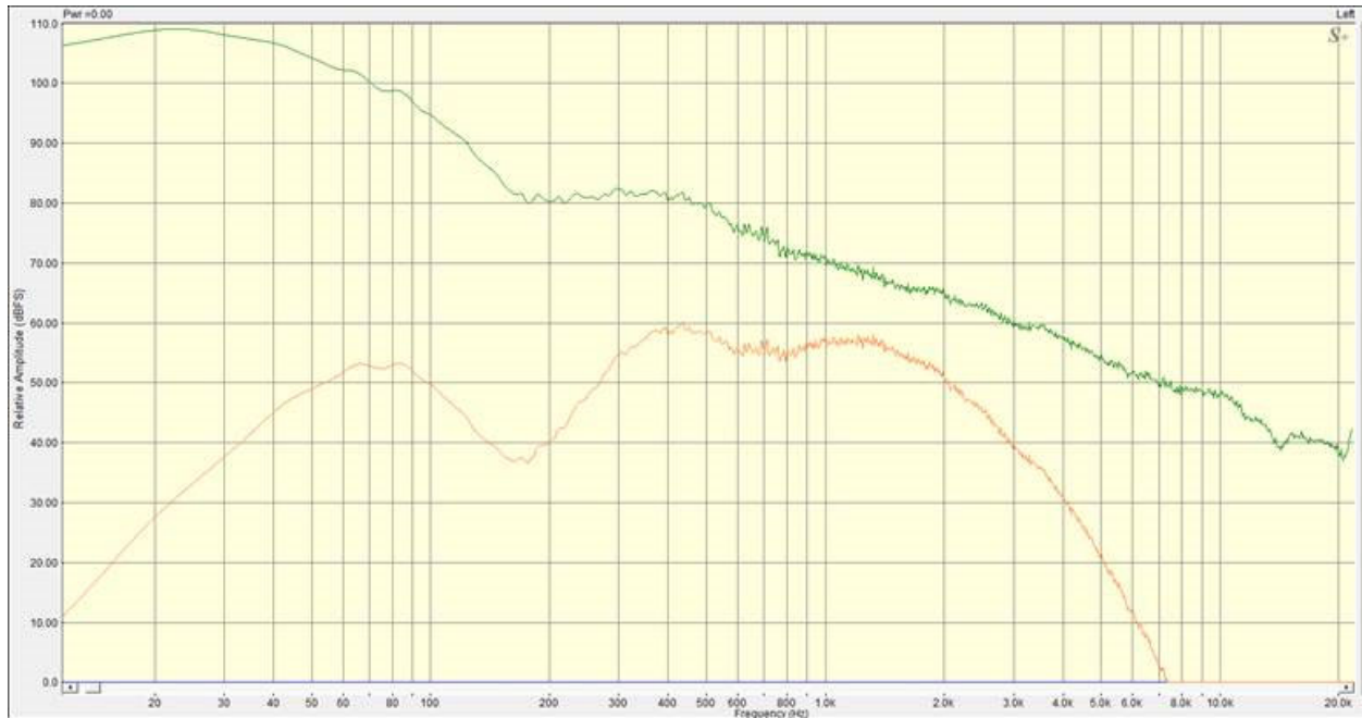
Figure 5.1-7. Launch peak noise level comparison of unweighted (green) versus SNPL-weighted (orange) decibels (note: time waveform recording from the June 2022 Falcon 9 SARah-1 launch).
