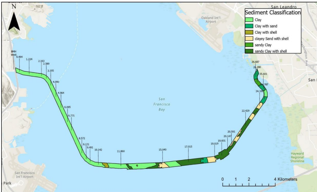
Figure 12: Bed Characterization along the Proposed Cable Route
