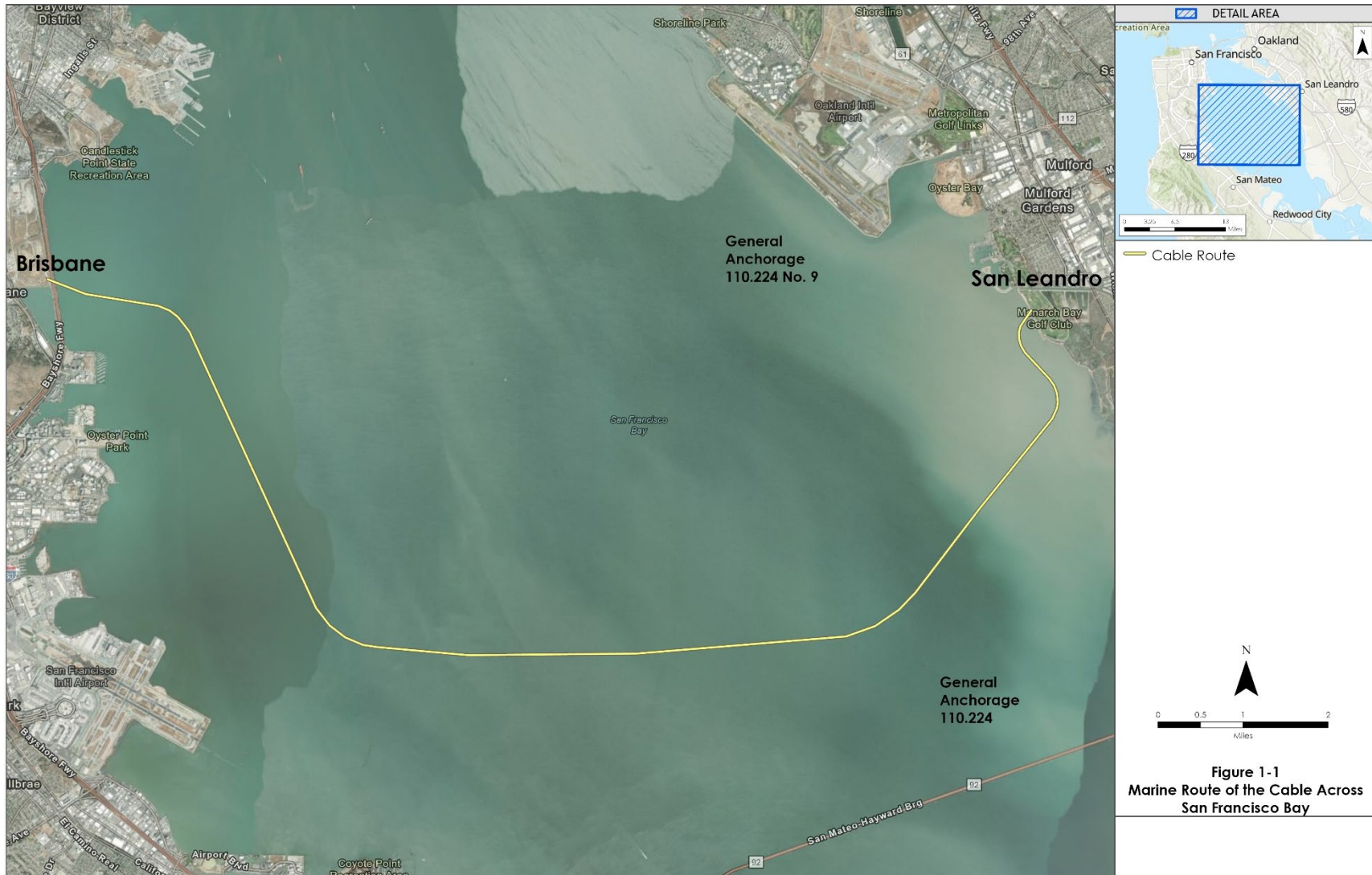
Figure 1-1. Marine Route of the Cables Across San Francisco Bay
