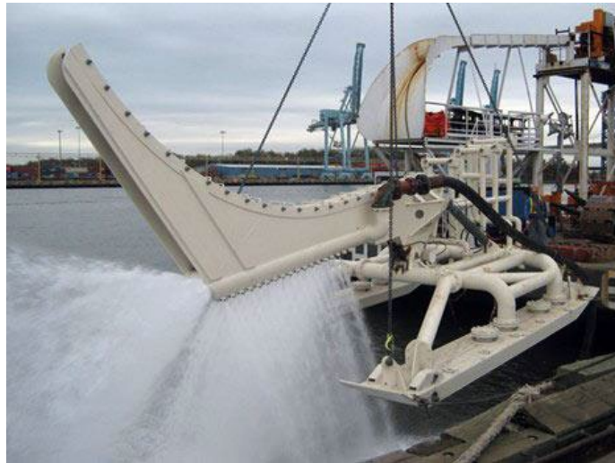
Figure 2.3-1. Surface-Powered Jetting Sled Burial Tool
