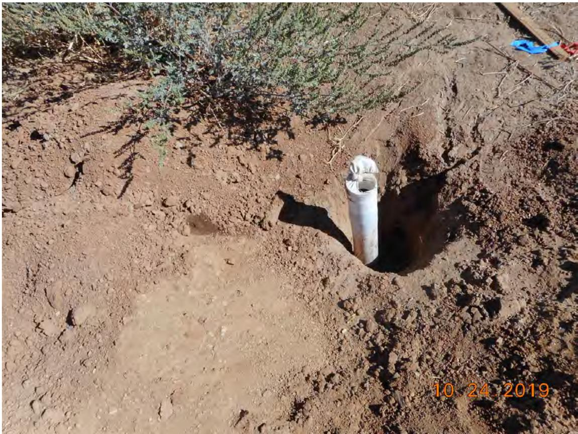
**Photo 11** - The infiltration test location shown is the southwesternmost onsite. To the left of the percolation pipe at this location is a small amount of oil-stained soil, as evidenced by the darker soil shown in the photograph.
