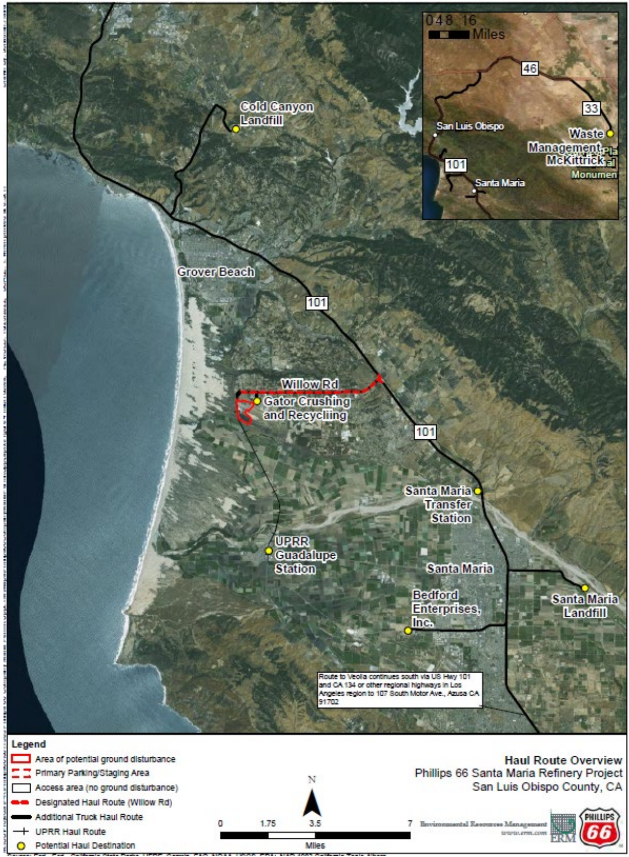
Figure 2 Offsite Haul Route and Potential Disposal/Transfer Locations
