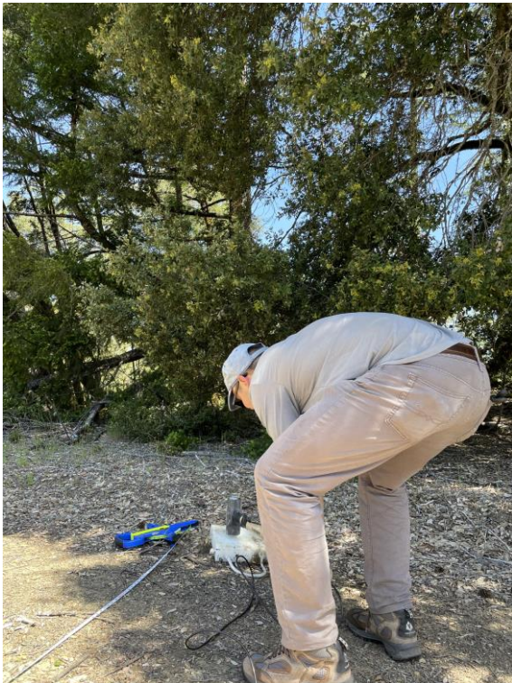
Figure 3 Surface wave testing at Location 2 ARGO-E LLC July 2022 La Doo Meadow, Briceland, CA
