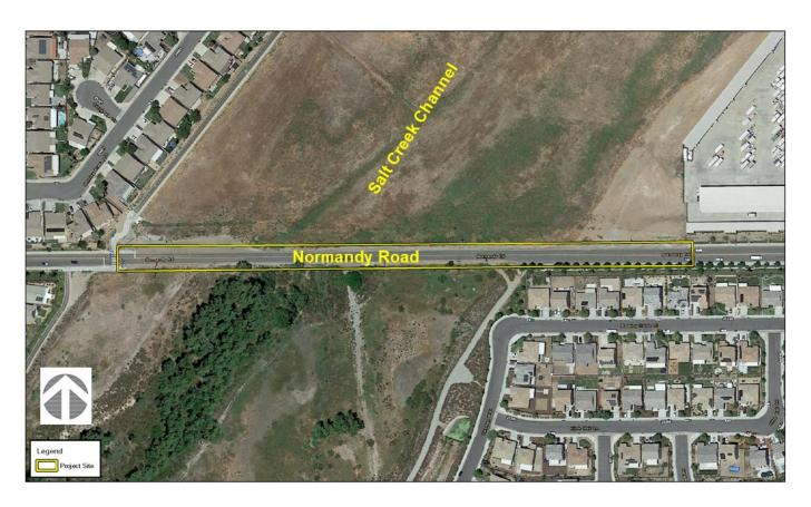
The City of Menifee (City) proposes the Normandy Road Pedestrian Improvements Project ("Project") which includes the construction of a pedestrian trail extending from existing sidewalks from the west and east along the north side of Normandy Road. The Project would include the demolition and grading of existing substrate, the construction of a pedestrian walkway, the installation of a pedestrian handrail and footing, site stabilization, striping of roadways, and final erosion mitigation.
