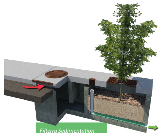
Filterra Sedimentation Chamber
