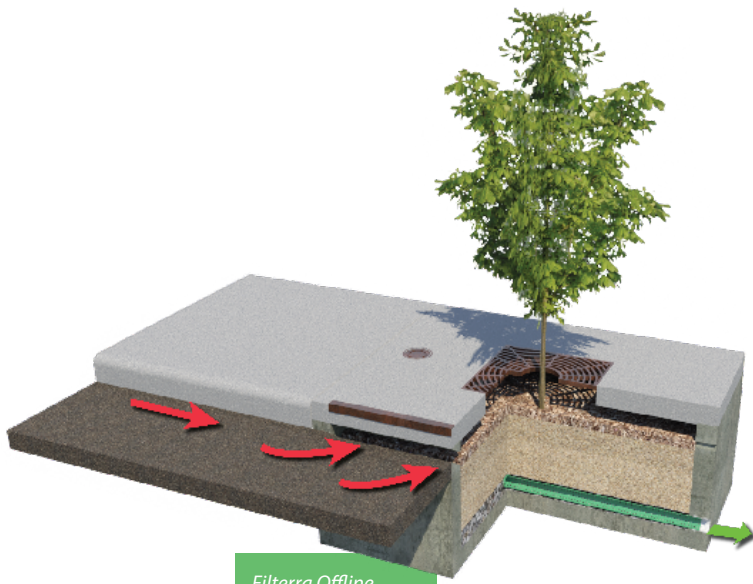
Filterra Offline Bypass via downstream catch basin.
