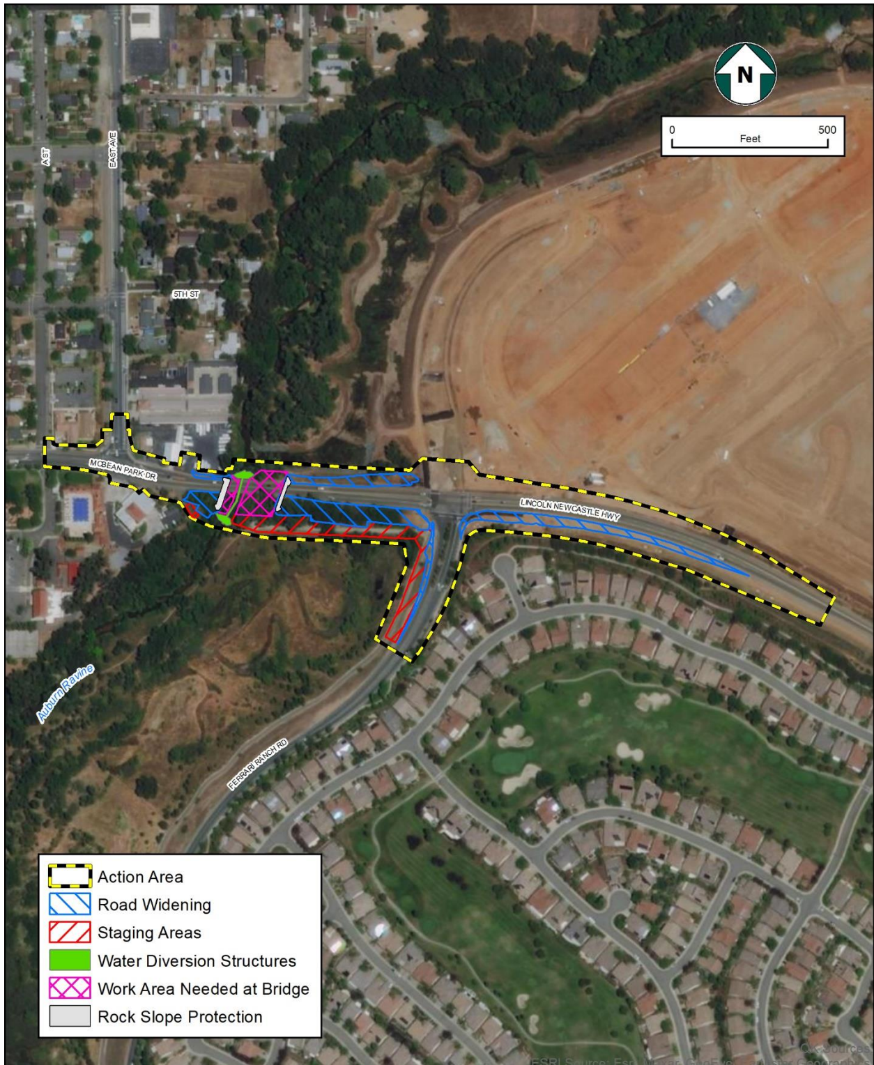
Figure 5 Project Footprint and Component Map McBean Park Drive Bridge Replacement Project, City of Lincoln, California
