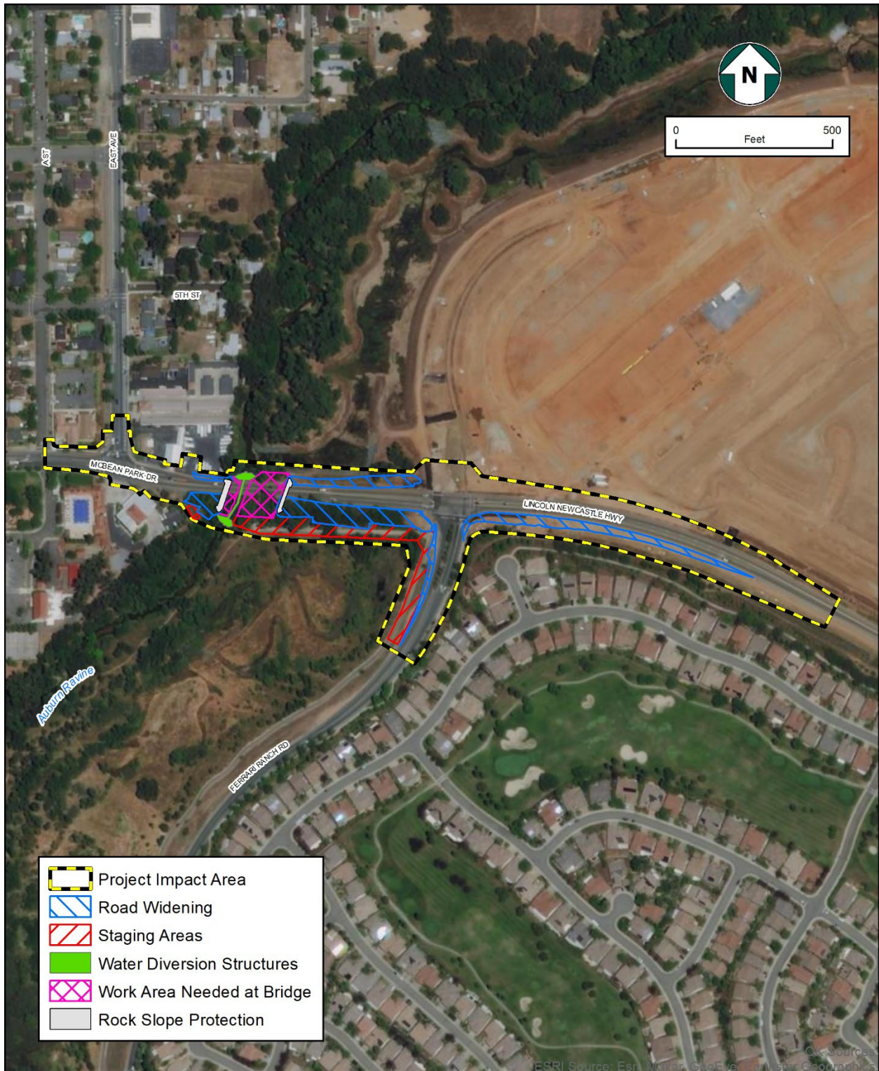
Figure 4 Project Impact Area and Project Component Map McBean Park Drive Bridge Replacement Project, City of Lincoln, California
