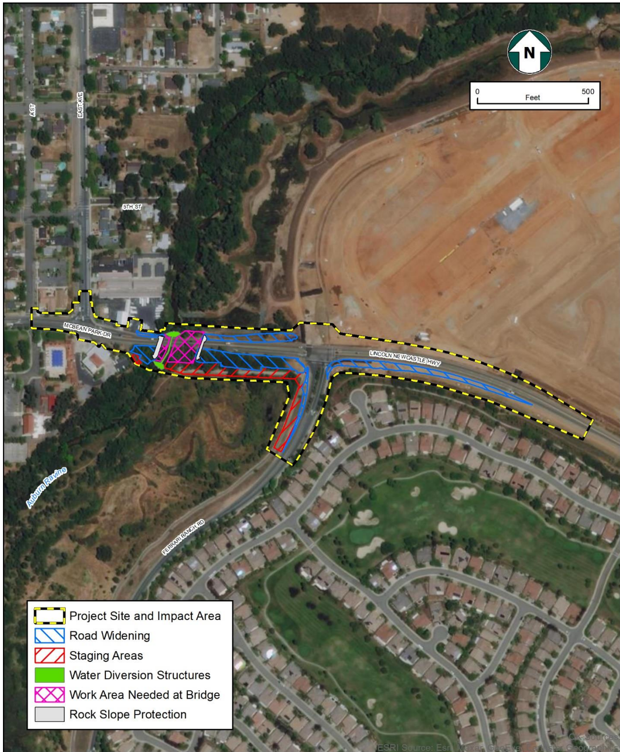
Figure 4 Project Footprint and Component Map, McBean Park Drive Bridge Replacement Project, City of Lincoln, California
