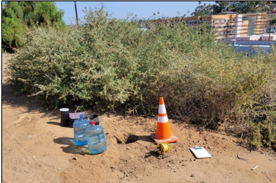
Figure 3-3. Percolation Testing, August 2021
