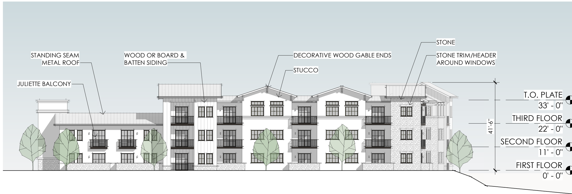
BUILDING A: WEST ELEVATION (FACING ALAMO PINTADO ROAD)
