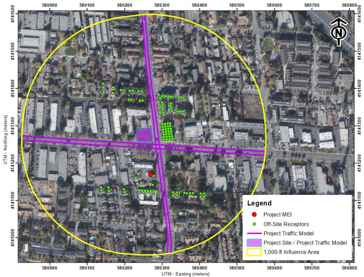
Figure 1. Locations of Project Construction Site, Project Traffic, Off-Site Sensitive Receptors, and Maximum TAC Impact
