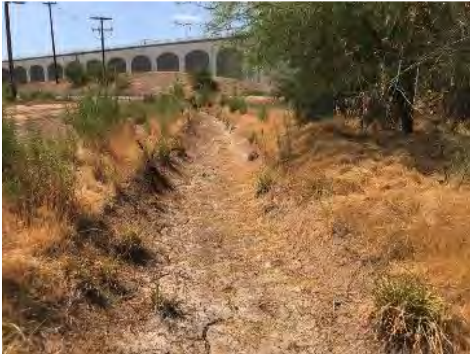
Photo 10. Upstream view of F2 at OHWM Data Point 2. The OHWM is defined by the presence of a break in slope with a bed and bank and change in vegetation cover and sediment. Photo taken facing north. July 18, 2018
