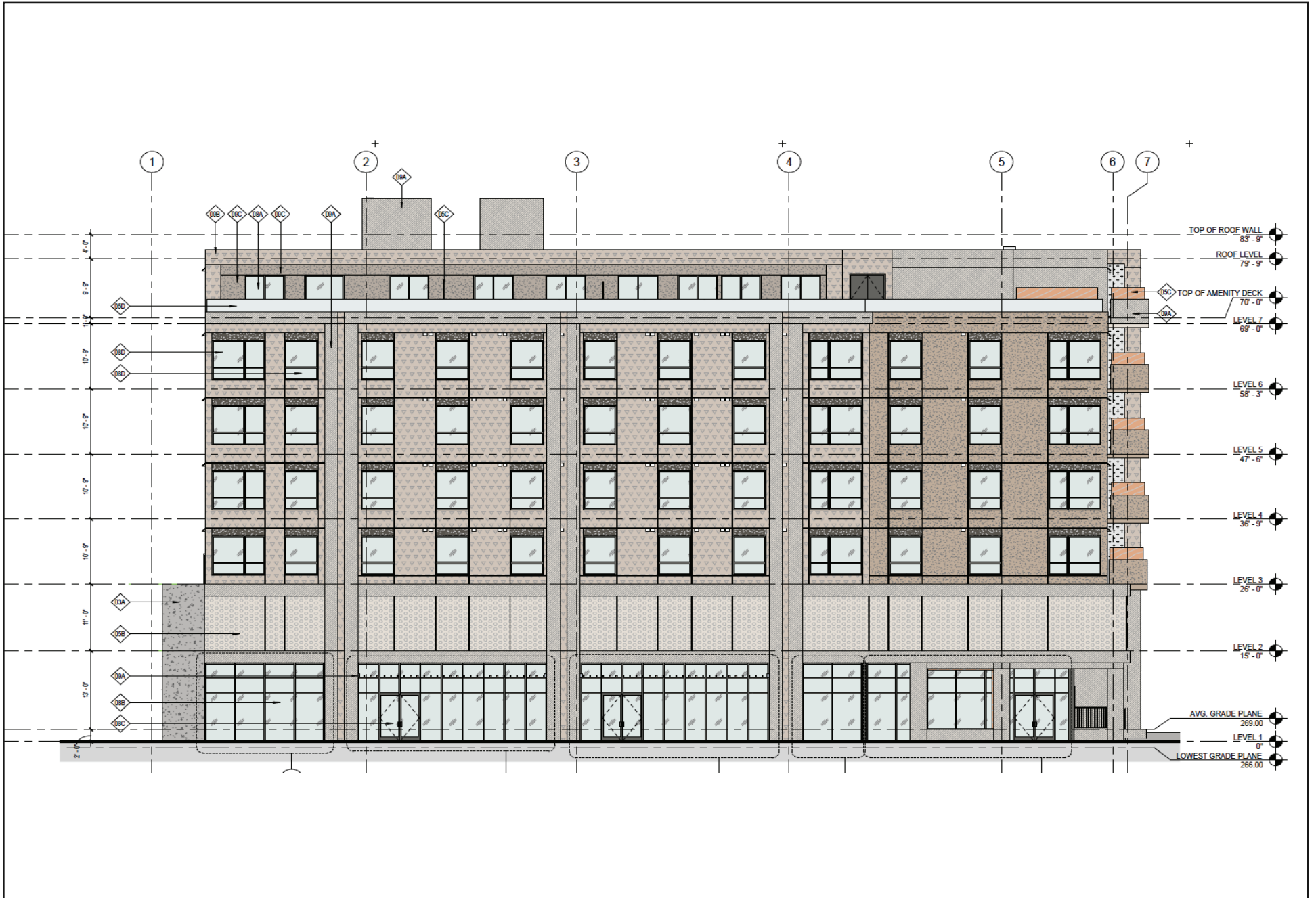
Figure 2.14 Building Elevation - South
